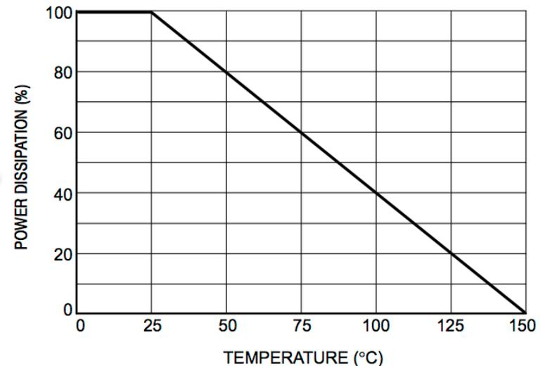
Figure 1. Steady State Power Derating
