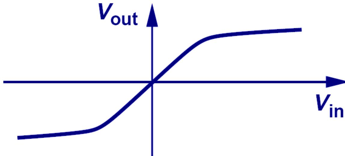
The clipping region is not exactly flat since as  $V_{in}$  increases, the currents through diodes change, and so does the voltage drop.
