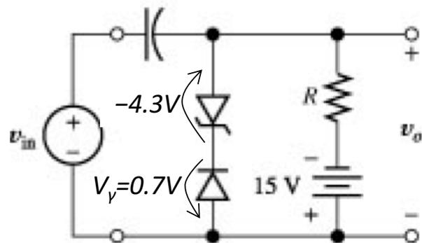
Circuit that clamps the negative peaks to  $-5V$
