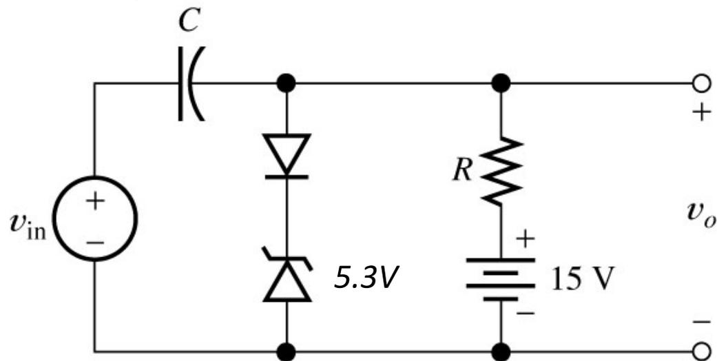
Circuit that clamps the positive peaks to +6V
