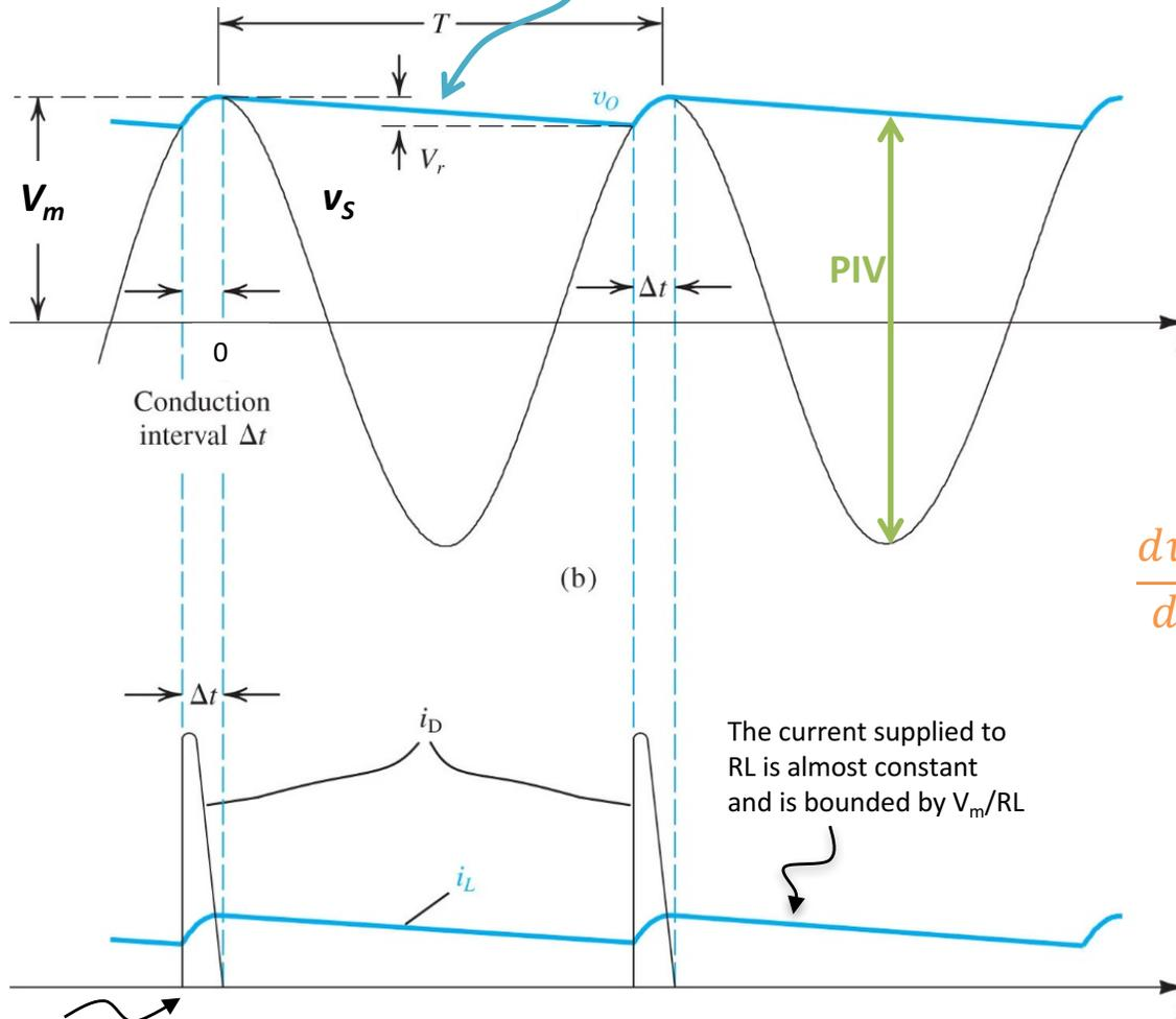
The diode's current is max at the beginning of the conduction interval and it goes down as the diode tends to turn off
