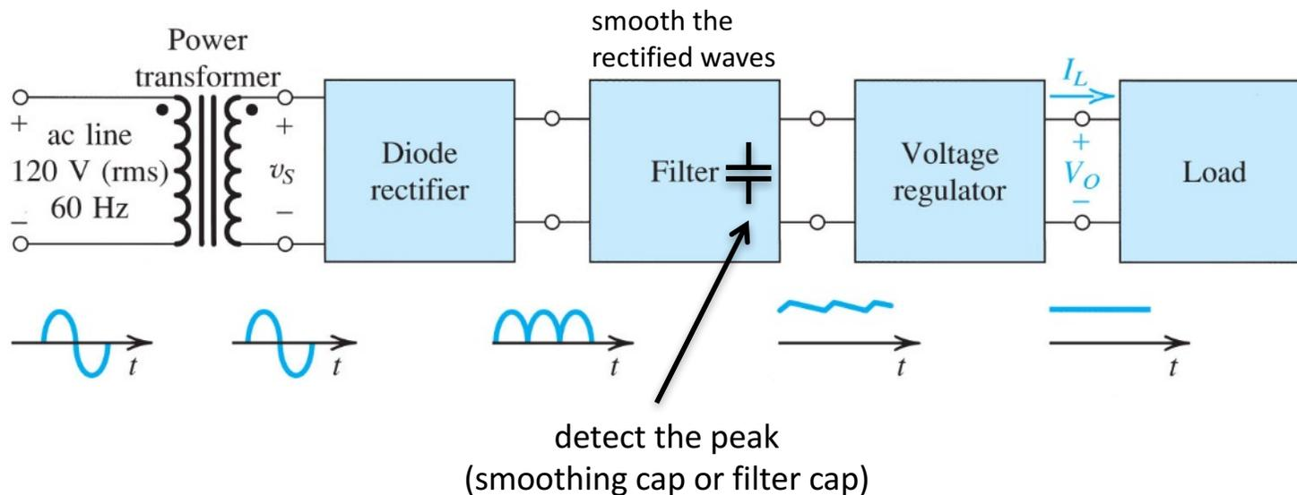
**Figure 4.22** Block diagram of a dc power supply.
