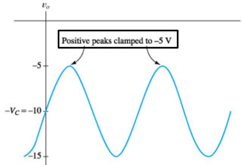
(b) Output waveform for  $v_{in} = 5 \sin(\omega t)$
