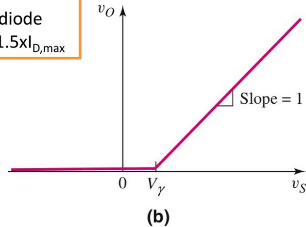
When the diode is ON
