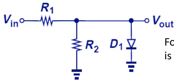
For  $V_{in} < 0$  the diode is definitely OFF
