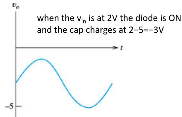
(b) Output for  $v_{in} = 2 \sin(\omega t)$
