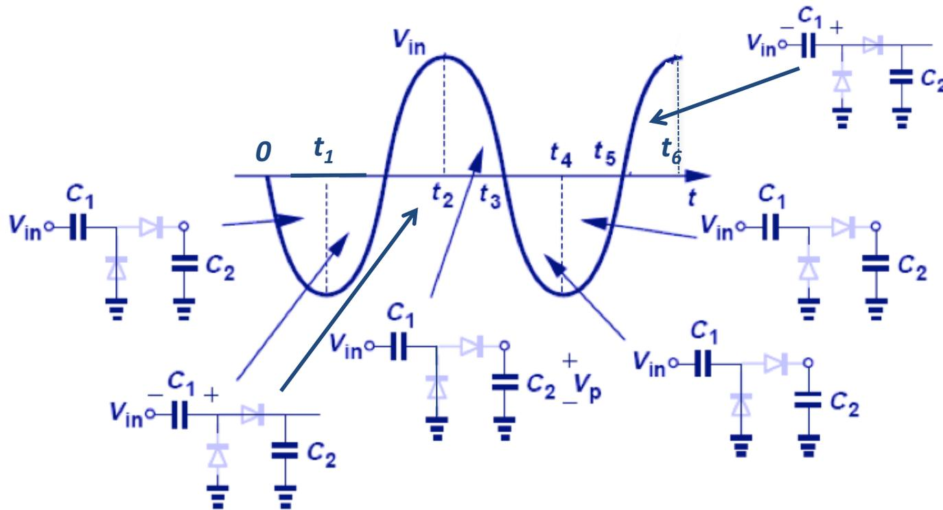
Each input cycle, the output increases by  $V_p$ ,  $V_p/2$ ,  $V_p/4$ , etc., eventually settling to  $2V_p$
