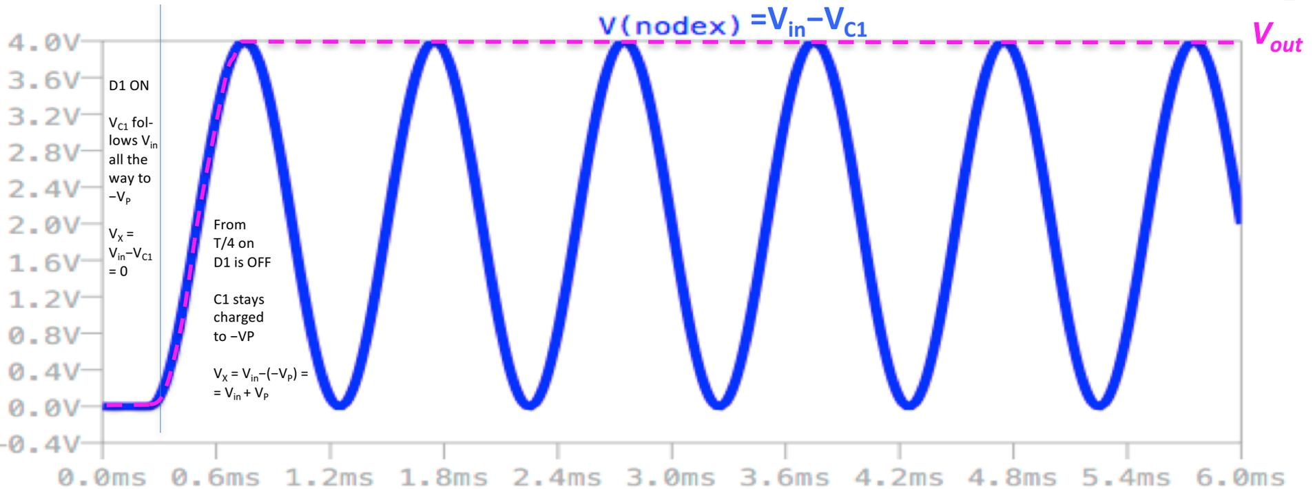
If we take the clamper just designed and attach a peak detector at its output we get a voltage doubler
