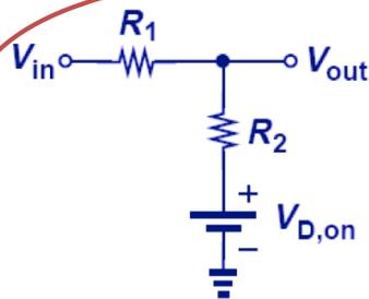
From the model of the circuit is easy to see that if  $V_{in} < V_{D,on}$  we cannot have current flowing through the diode  $\Rightarrow$  the diode must be **OFF**  $\rightarrow V_{out} = V_{in}$
