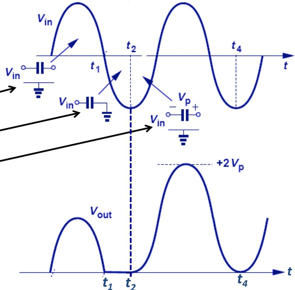
The negative peaks of the output voltage are clamped at 0 V
