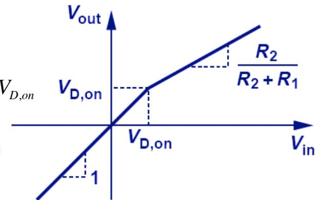
When the diode is **ON** we can model the circuit as follow:
