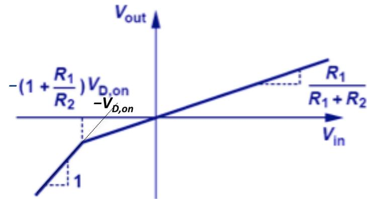
For  $V_{in} < 0$  the diode is definitely ON.
