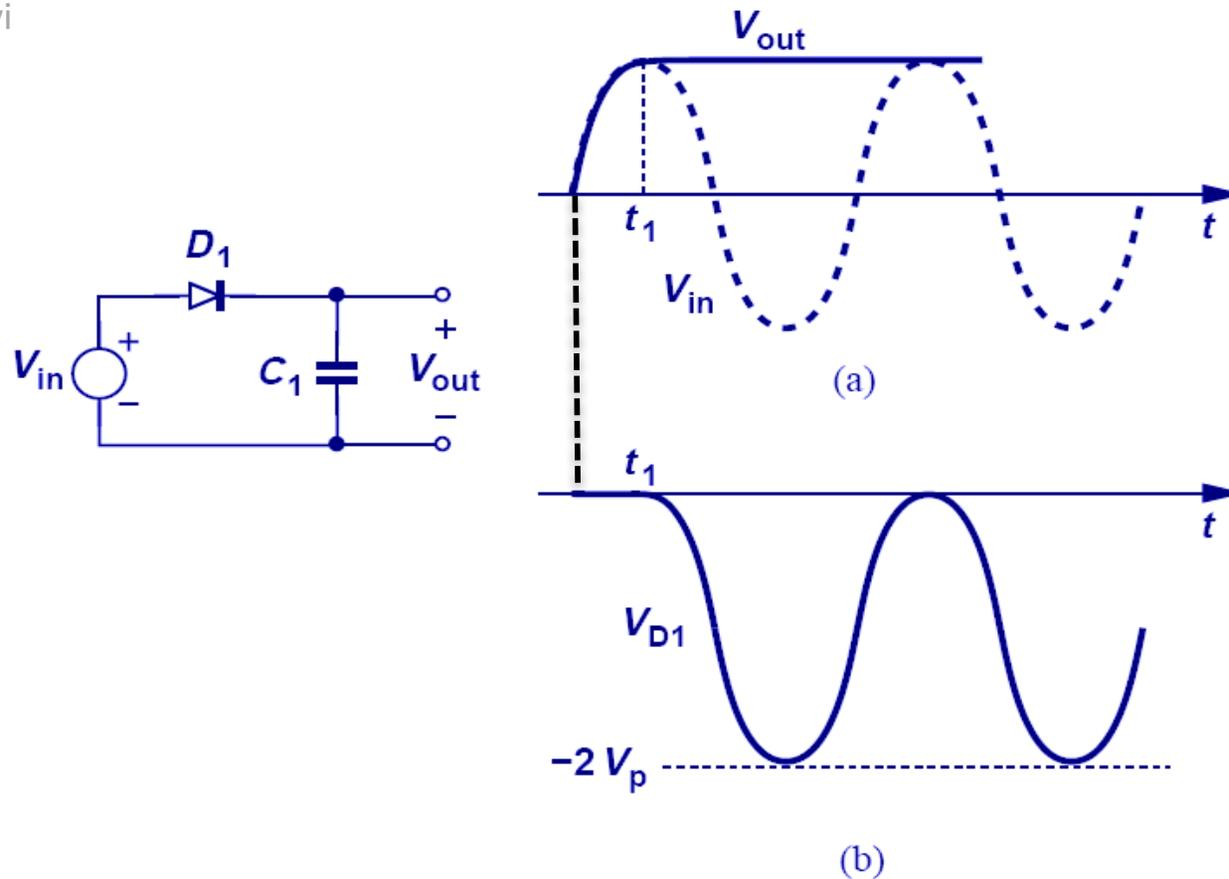
Note: the voltage across the diode ( $V_{D1}$ ) is just like  $V_{in}$ , only shifted down
