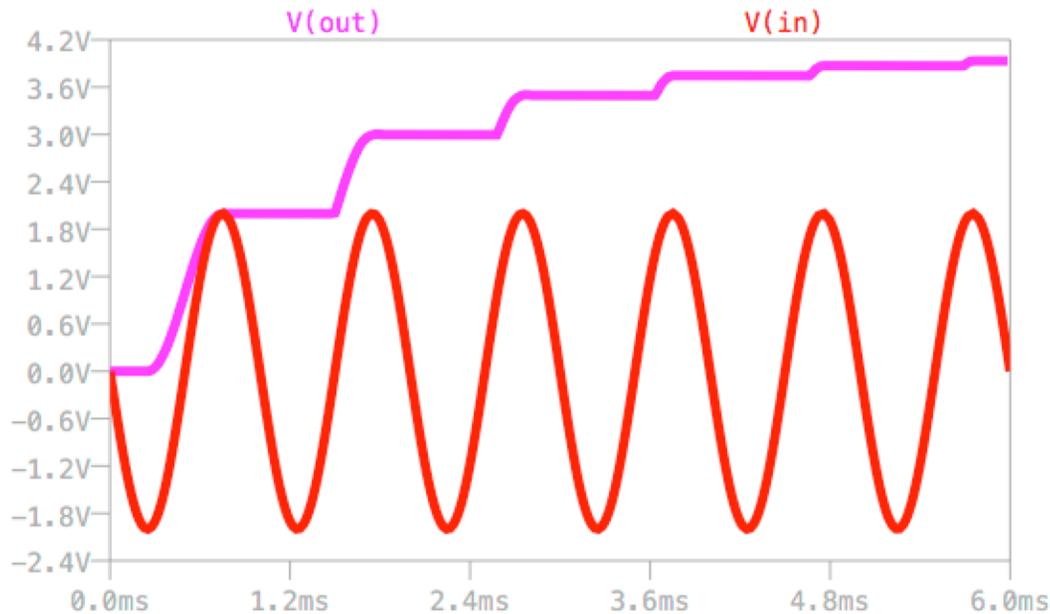
In the reality the charging of  $C_1$  and  $C_2$  ( $V_{C_2} = V_{out}$ ) is not as simple as assumed in the previous slide (slide 52 is a snapshot of the steady state)
