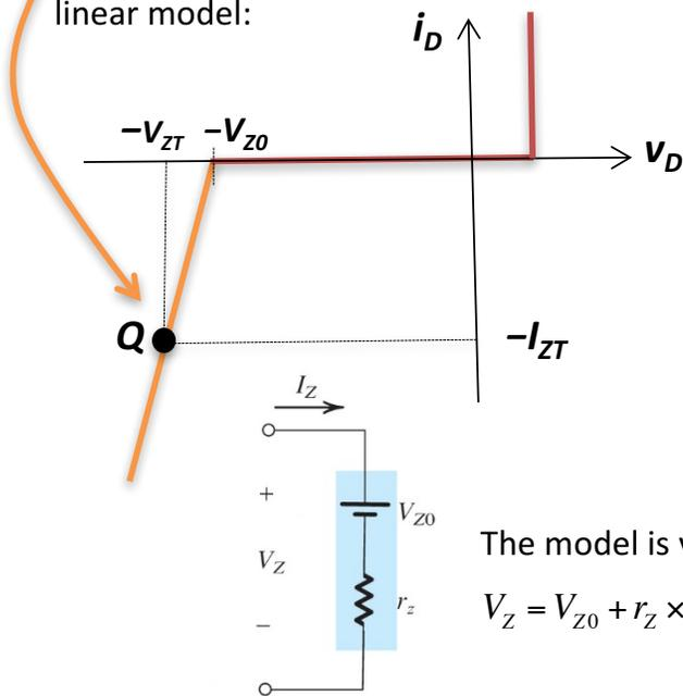
The model is valid for  $I_Z > I_{ZK}$  and  $V_Z > V_{Z0}$ :
