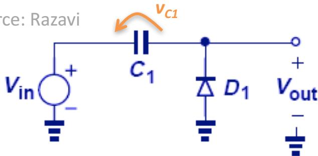
initially the cap is uncharged:  $v_{C1}(0)=0$
