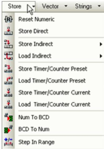
2. Select **Reset Numeric**, then place the function in the desired net. In the following picture, when MB 0 turns ON, MI 0 = 0.
