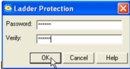
2. To apply the password to a subroutine, right-click the subroutine's name in the Project Navigation window, then select Set as Protected; a small padlock icon is displayed next to the subroutine's name. You can also right-click a module's name and select Protect All Subroutines in Module.
