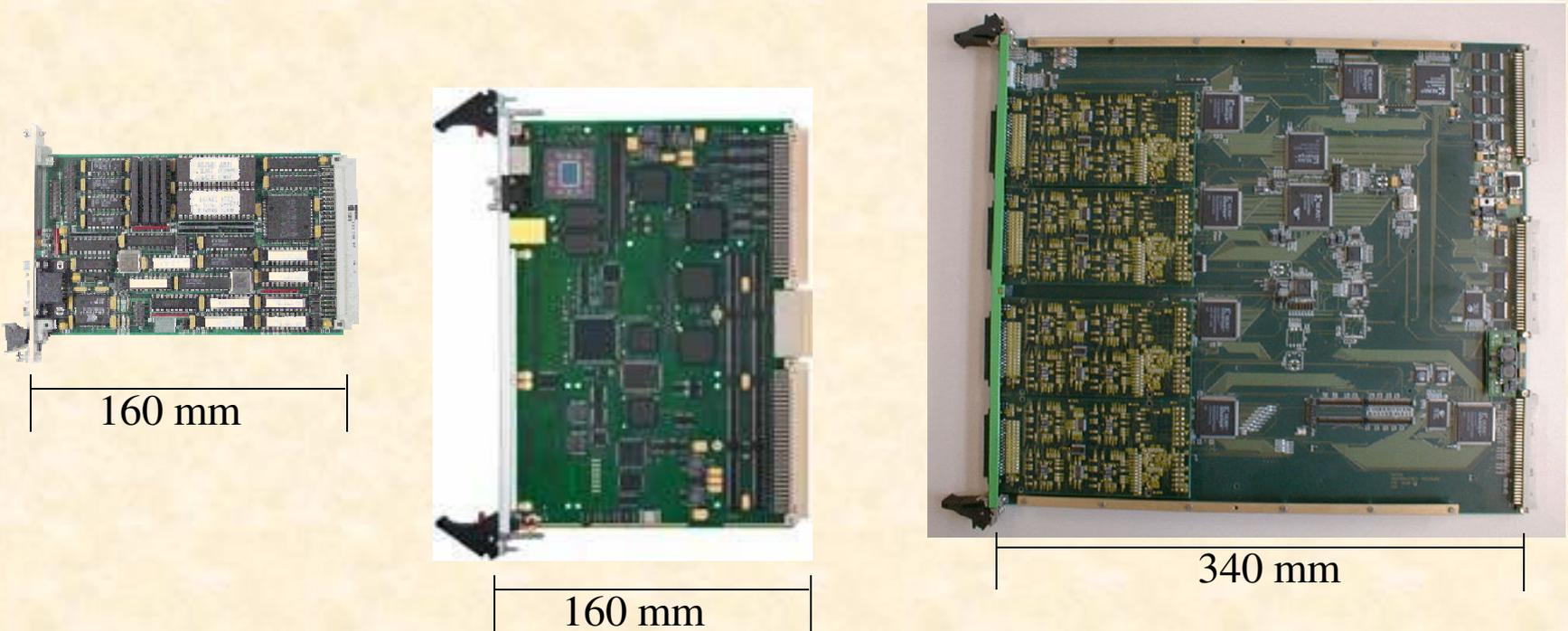
In 6U and 9U systems there can be transition modules installed on the rear side of the backplane. Transition modules do not connect to VMEbus but just to the VMEbus module on the opposite side of the backplane via the user defined pins of the J0, J2 and J3 connectors
