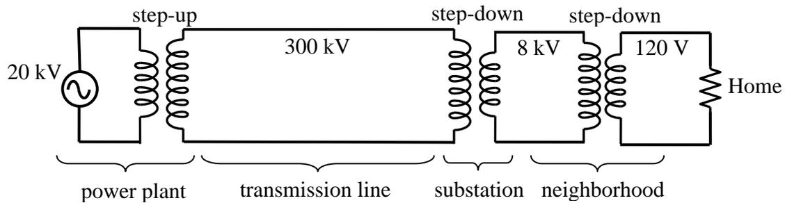
A very simplified model of power distribution (transformers not shown):
