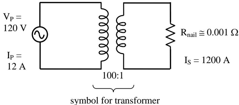
Power dissipated in nail =  $I_S^2 R = (1200)^2 (10^{-3}) = 1440 \text{ W} \Rightarrow$  will melt nail.
