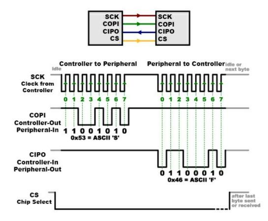
The CS line is normally held high, which disconnects the peripheral from the SPI bus. (This type of logic is known as "active low," and you'll often see used it for enable and reset lines.) Just before data is sent to the peripheral, the line is brought low, which activates the peripheral. When you're done using the peripheral, the line is made high again. In a <u>shift register</u>, this corresponds to the "latch" input, which transfers the received data to the output lines.
