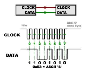
One reason that SPI is so popular is that the receiving hardware can be a simple<u>shift register</u>. This is a much simpler (and cheaper!) piece of hardware than the full-up UART (Universal Asynchronous Receiver / Transmitter) that asynchronous serial requires.
