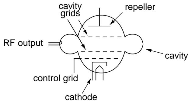
As a voltage-controlled oscillator, reflex klystron tubes served commonly as "local oscillators" for radar equipment and microwave receivers:
