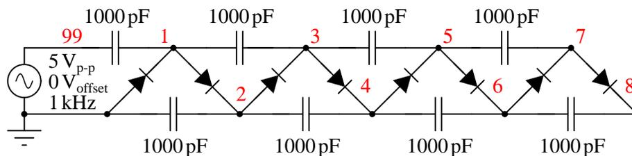
Figure 3.48: *Cockcroft-Walton* x8 voltage multiplier; output at v(8).
