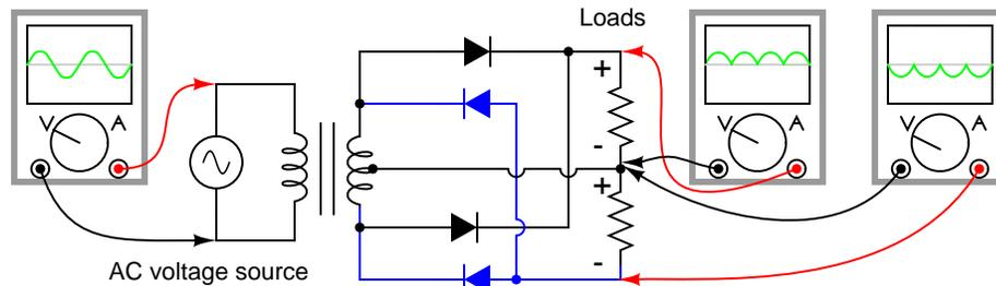
Figure 3.19: *Dual polarity full-wave center tap rectifier*
