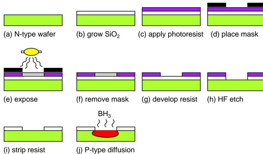
Figure 2.54: *Manufacture of a silicon diode junction.*
