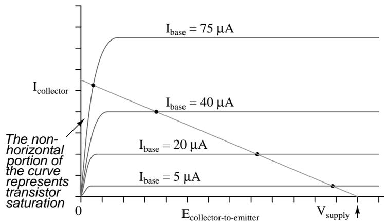
Figure 4.73: Load line resulting from increased load resistance.
