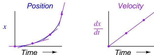
What does this have to do with analog electronic circuits? Well, if we were to have an analog voltage signal represent the car's position (think of a huge potentiometer whose wiper was attached to the car, generating a voltage proportional to the car's position), we could connect a differentiator circuit to this signal and have the circuit continuously *calculate* the car's velocity, displaying the result via a voltmeter connected to the differentiator circuit's output:
