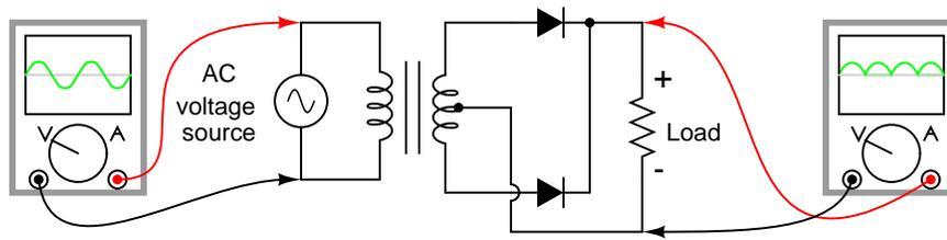
Figure 3.16: Full-wave rectifier, center-tapped design.
