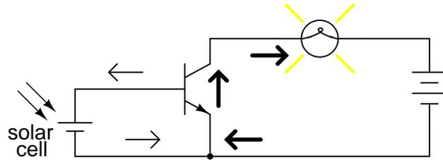
Figure 4.5: Solar cell serves as light sensor.
