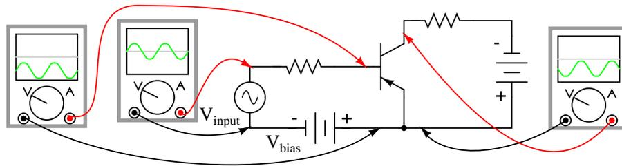
Figure 4.38: PNP version of common emitter amplifier.
