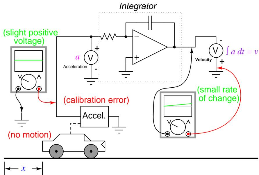
As with differentiation, this error will also compound itself if the integrated signal is passed on to another integrator circuit, since the "drifting" output of the first integrator will very soon present a significant positive or negative signal for the next integrator to integrate. Therefore, care should be taken when integrating sensor signals: if the "zero" adjustment of the sensor is not *perfect*, the integrated result will drift, even if the integrator circuit itself is perfect.
