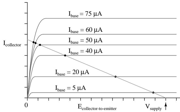
Figure 4.74: More base current curves shows saturation detail.
