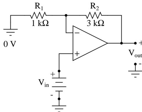
Inverting op-amp circuits may be modeled using the lever analogy as well. With the inverting configuration, the ground point of the feedback voltage divider is the op-amp's inverting input with the input to the left and the output to the right. This is mechanically equivalent to a *first-class* lever, where the input force (effort) is on the opposite side of the fulcrum from the output (load):
