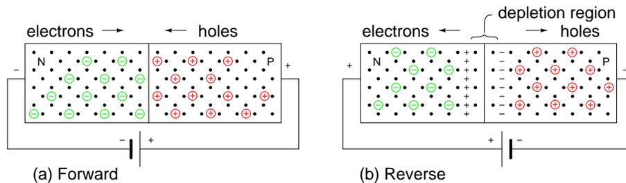
Figure 2.29: (a) *Forward battery bias repels carriers toward junction, where recombination results in battery current.* (b) *Reverse battery bias attracts carriers toward battery terminals, away from junction. Depletion region thickness increases. No sustained battery current flows.*
