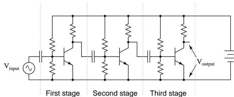
Figure 4.101: *Capacitor coupled three stage common-emitter amplifier.*
