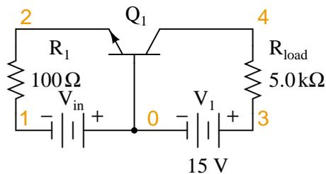
Figure 4.54: Common-base circuit for DC SPICE analysis.
