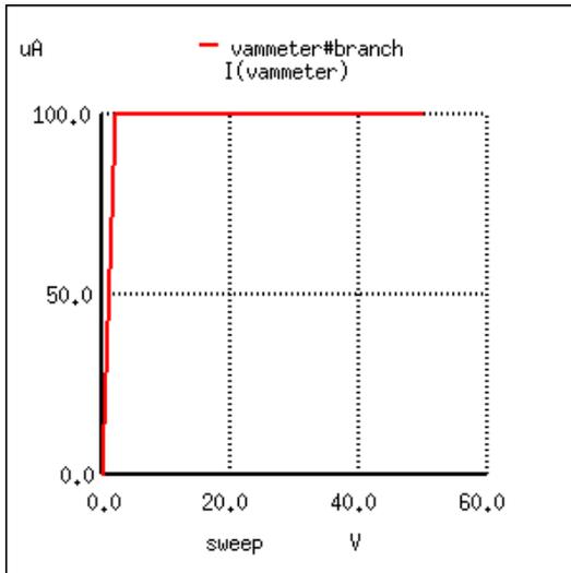
Sure enough, the drain current remains steady at a value of  $100 \mu\text{A}$  ( $1.000\text{E-}04$  amps) no matter how high the power supply voltage is adjusted.
