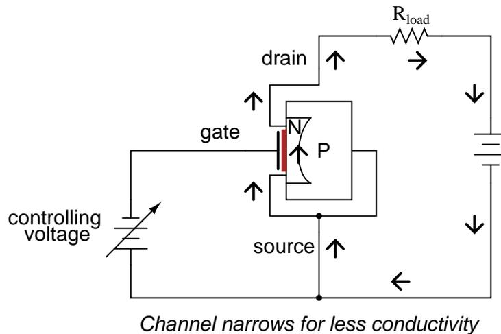
The insulated gate allows for controlling voltages of any polarity without danger of forward-biasing a junction, as was the concern with JFETs. This type of IGFET, although its called a "depletion-type," actually has the capability of having its channel *either* depleted (channel narrowed) *or* enhanced (channel expanded). Input voltage polarity determines which way the channel will be influenced.
