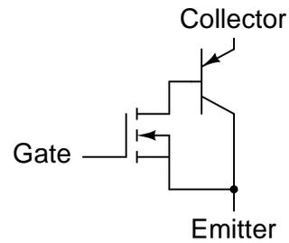
In essence, the IGFET controls the base current of a BJT, which handles the main load current between collector and emitter. This way, there is extremely high current gain (since the insulated gate of the IGFET draws practically no current from the control circuitry), but the collector-to-emitter voltage drop during full conduction is as low as that of an ordinary BJT.
