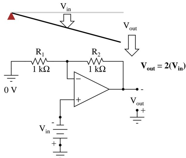
If we alter the resistor ratio  $R_2/R_1$ , we change the gain of the op-amp circuit. In lever terms, this means moving the input point in relation to the fulcrum and lever end, which similarly changes the displacement "gain" of the machine:
