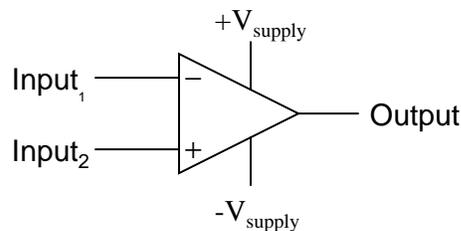
The two input leads can be seen on the left-hand side of the triangular amplifier symbol, the output lead on the right-hand side, and the +V and -V power supply leads on top and bottom. As with the other example, all voltages are referenced to the circuit's ground point. Notice that one input lead is marked with a (-) and the other is marked with a (+). Because a differential amplifier amplifies the difference in voltage between the two inputs, each input influences the
