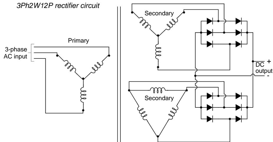
Figure 3.27: Polyphase rectifier circuit: 3-phase 2-way 12-pulse (3Ph2W12P)
