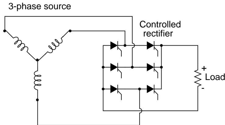
Figure 7.38: Three-phase bridge SCR control of load
