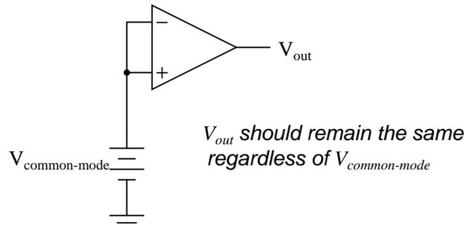
Voltage that is common between either of the inputs and ground, as " $V_{common-mode}$ " is in this case, is called *common-mode voltage*. As we vary this common voltage, the perfect differential amplifier's output voltage should hold absolutely steady (no change in output for any arbitrary change in common-mode input). This translates to a *common-mode voltage gain* of zero.
