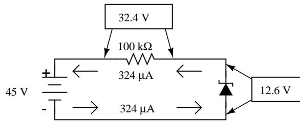
Figure 3.60: Zener regulator with 100 kΩ resistor.
