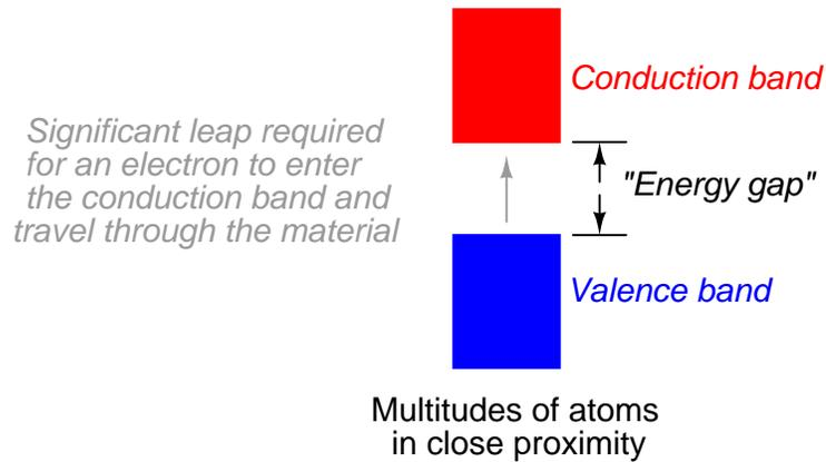
Figure 2.21: *Electron band separation in insulating substances.*
