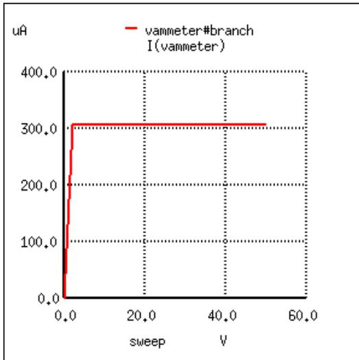
With the gate-source voltage set to 0.25 volts, one-half what it was before, the drain current is  $306.3 \mu\text{A}$ . Although this is still an increase over the  $225 \mu\text{A}$  from the prior simulation, it isn't *proportional* to the change of the controlling voltage.
