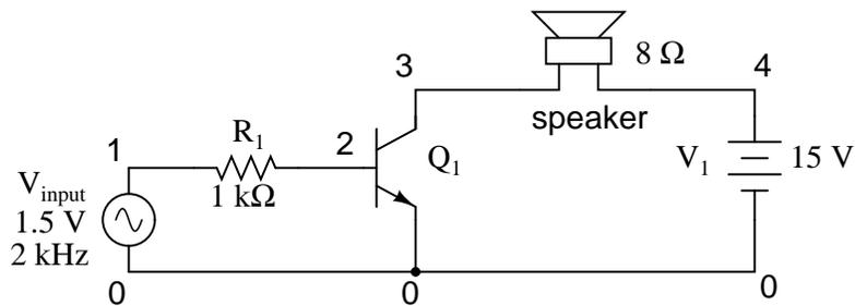
Figure 4.29: SPICE version of common emitter audio amplifier.
