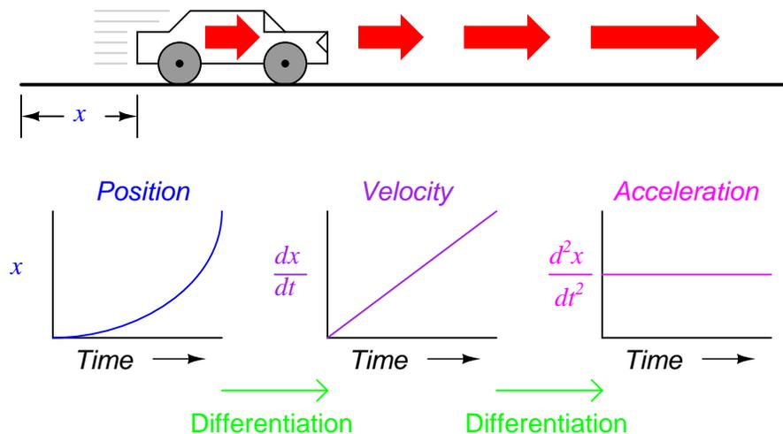
The expression  $d^2x/dt^2$  is called the *second derivative* of position ( $x$ ) with regard to time ( $t$ ). If we were to connect a second differentiator circuit to the output of the first, the last voltmeter would register acceleration:
