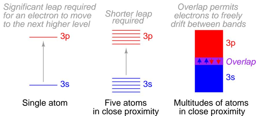
Figure 2.20: *Electron band overlap in metallic elements.*
