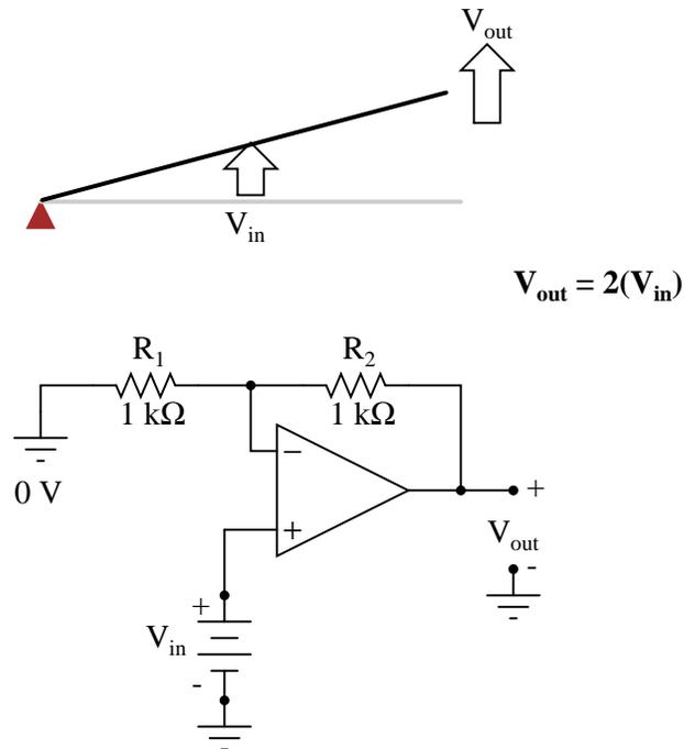
Due to the displacement-amplifying characteristics of the lever, the "output" point will move twice as far as the "input" point, and in the same direction. In the electronic circuit, the output voltage will equal twice the input, with the same polarity. Applying a negative input voltage is analogous to moving the lever downward from its level "zero" position, resulting in an amplified output displacement that is also negative:
