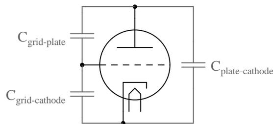
Now, this stray capacitance is quite small, and the reactive impedances usually high. Usually, that is, unless radio frequencies are being dealt with. As we saw with De Forest's Audion tube, radio was probably the prime application for this new technology, so these "tiny" capacitances became more than just a potential problem. Another refinement in tube technology was necessary to overcome the limitations of the triode.
