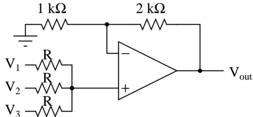
With a voltage divider composed of a 2 kΩ / 1 kΩ combination, the noninverting amplifier circuit will have a voltage gain of 3. By taking the voltage from the passive averager, which is the sum of  $V_1$ ,  $V_2$ , and  $V_3$  divided by 3, and multiplying that average by 3, we arrive at an output voltage equal to the *sum* of  $V_1$ ,  $V_2$ , and  $V_3$ :
