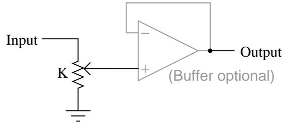
$$\text{Output} = \frac{\text{Input}}{K}$$
