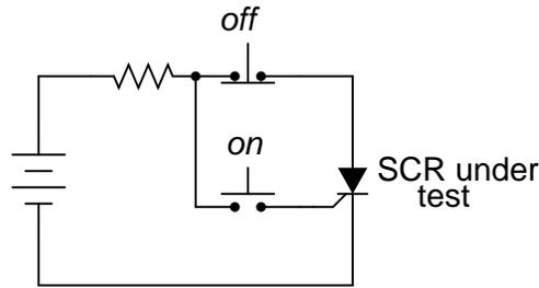
Figure 7.23: SCR testing circuit
