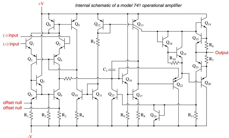
Figure 8.7: Schematic diagram of a model 741 op-amp.
