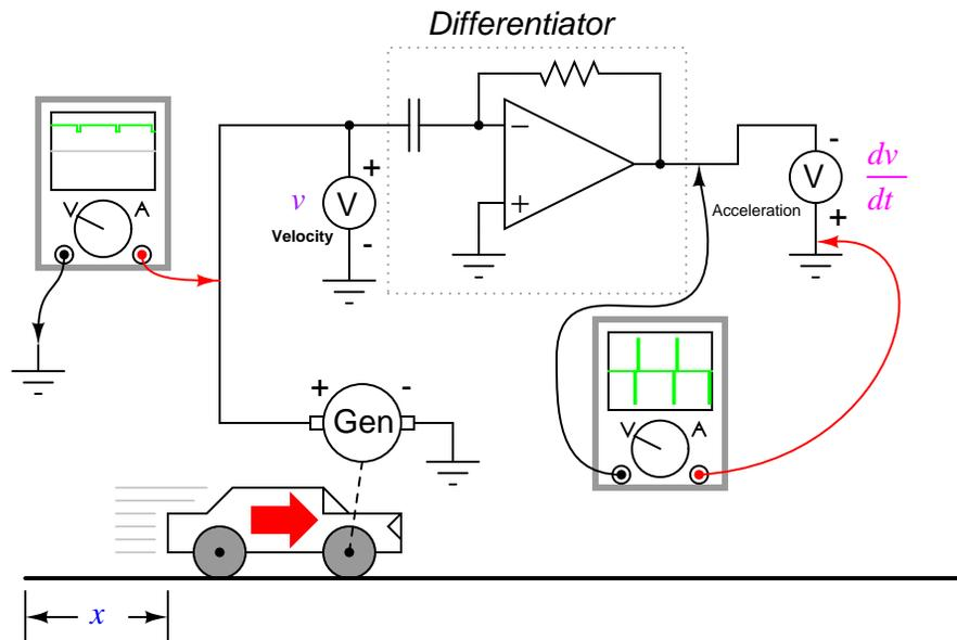
Noise voltage present in a signal to be differentiated need not be of significant amplitude to cause trouble: all that is required is that the noise profile have fast rise or fall times. In other words, any electrical noise with a high  $dv/dt$  component will be problematic when differentiated, even if it is of low amplitude.
