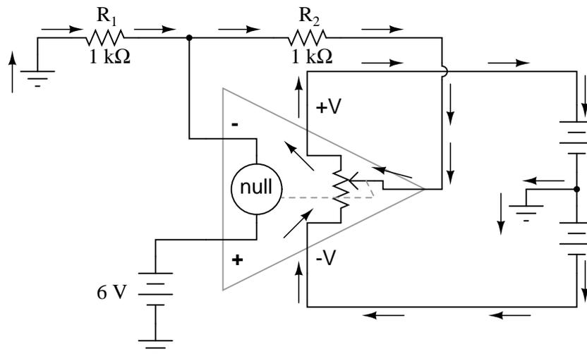
Here, arrows denote the path of electron flow through the power supply batteries, both for powering the op-amp's internal circuitry (the "potentiometer" inside of it that controls output
