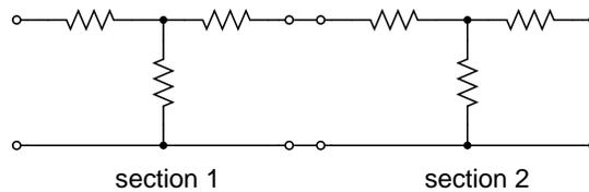
Figure 1.19: Cascaded attenuator sections: dB attenuation is additive.
