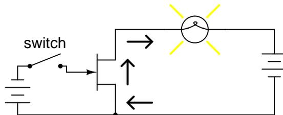
Closing this switch will "pinch off" the JFET's channel, thus forcing it into cutoff and turning the lamp off:
