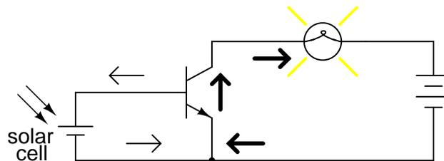
Figure 4.20: NPN transistor as a simple switch.
