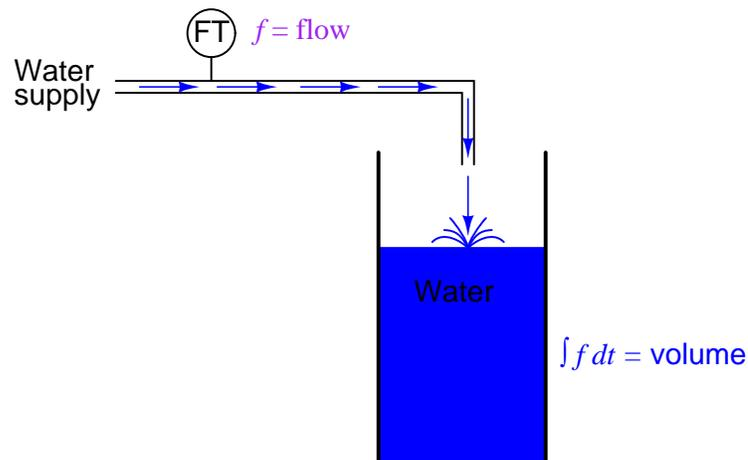
If we were to use a "Flow Transmitter" device to measure water flow, then by time-integration we could calculate the volume of water accumulated in the tank over time. Although it is theoretically possible to use a capacitive op-amp integrator circuit to derive a volume signal from a flow signal, mechanical and digital electronic "integrator" devices are more suitable for integration over long periods of time, and find frequent use in the water treatment and distribution industries.
