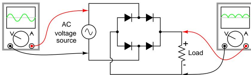
Figure 3.23: Alternative layout style for Full-wave bridge rectifier.
