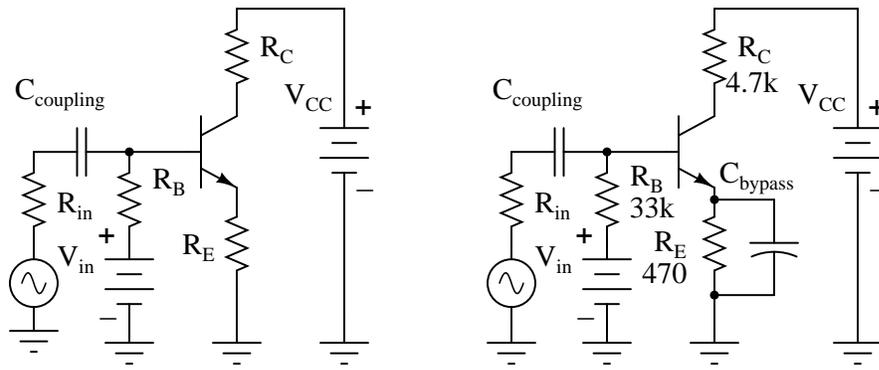
Figure 4.89: *C<sub>bypass</sub>* is required to prevent AC gain reduction.
