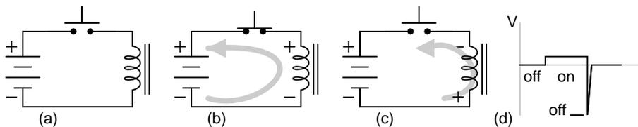
Figure 3.50: *Inductive kickback: (a) Switch open. (b) Switch closed, electron current flows from battery through coil which has polarity matching battery. Magnetic field stores energy. (c) Switch open, Current still flows in coil due to collapsing magnetic field. Note polarity change on coil. (d) Coil voltage vs time.*
