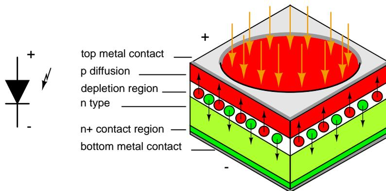
Figure 3.74: *Photodiode: Schematic symbol and cross section.*
