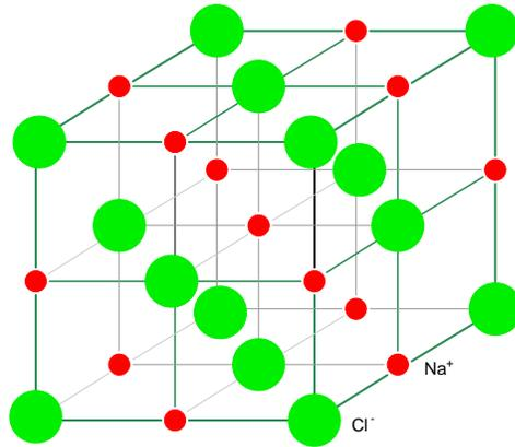
Figure 2.16: NaCl crystal having a cubic structure.
