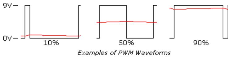
The reason PWM is popular is simple. Many loads, such as resistors, integrate the power into a number matching the percentage. Conversion into its analog equivalent value is straightforward. LEDs are very nonlinear in their response to current, give an LED half its rated current you still get more than half the light the LED can produce. With PWM the light level produced by the LED is very linear. Motors, which will be covered later, are also very responsive to PWM.
