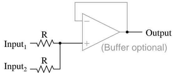
$$\text{Output} = \frac{\text{Input}_1 + \text{Input}_2}{2}$$
