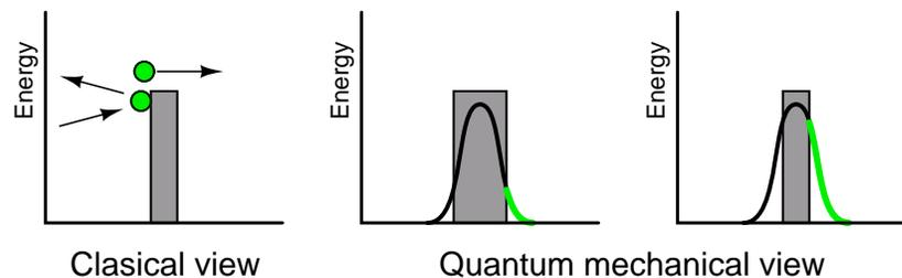
Figure 2.58: *Classical view of an electron surmounting a barrier, or not. Quantum mechanical view allows an electron to tunnel through a barrier. The probability (green) is related to the barrier thickness. After Figure 1 [22]*
