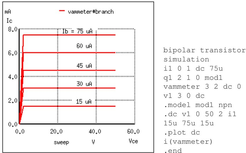
Figure 4.16: Sweeping collector voltage 0 to 50 V (.dc v1 0 50 2) with base current constant at  $75\ \mu\text{A}$  yields constant 7.5 mA collector current. Other curves are generated by current sweep (i1 15u 75u 15u) in DC analysis statement (.dc v1 0 50 2 i1 15u 75u 15u).
