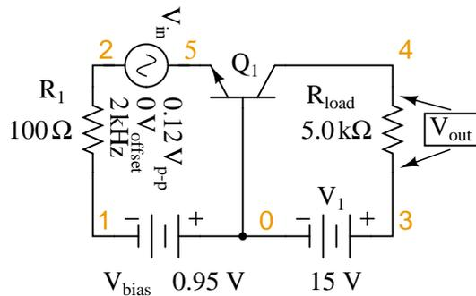
Figure 4.56: Common-base circuit for SPICE AC analysis.
