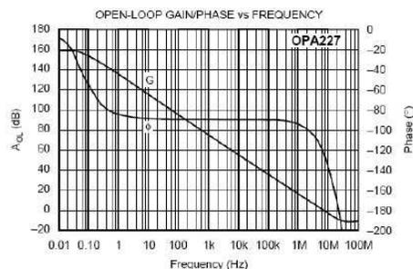
Figure 8.2:  $A_V$  and  $\Phi$  vs. Frequency plot
