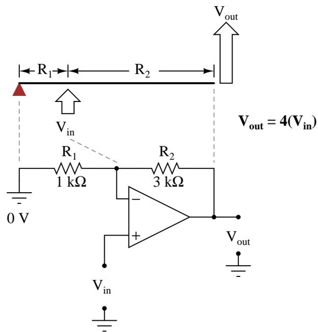
Now, any input signal will become amplified by a factor of four instead of by a factor of two:
