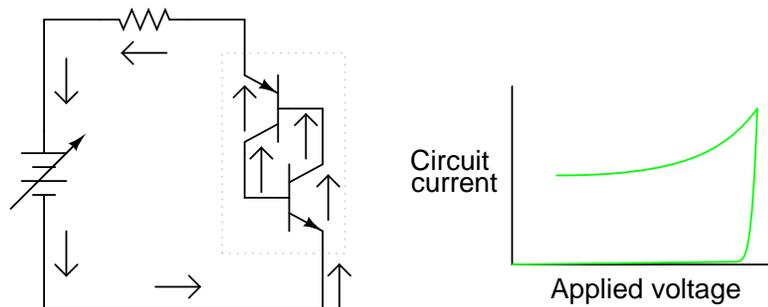
Figure 7.13: *Current maintained even when voltage is reduced*
