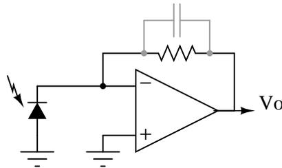
Figure 9.25: Photodiode amplifier.
