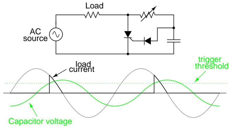
Figure 7.33: Phase-shifted signal triggers SCR into conduction.
