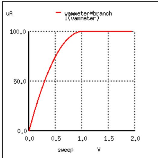
Here, the controlling signal is a steady voltage of 1 volt, applied with negative towards the JFET gate and positive toward the JFET source, to reverse-bias the PN junction. In the first BJT simulation of chapter 4, a constant-current source of  $20 \mu\text{A}$  was used for the controlling signal, but remember that a JFET is a *voltage-controlled* device, not a current-controlled device like the bipolar junction transistor.
