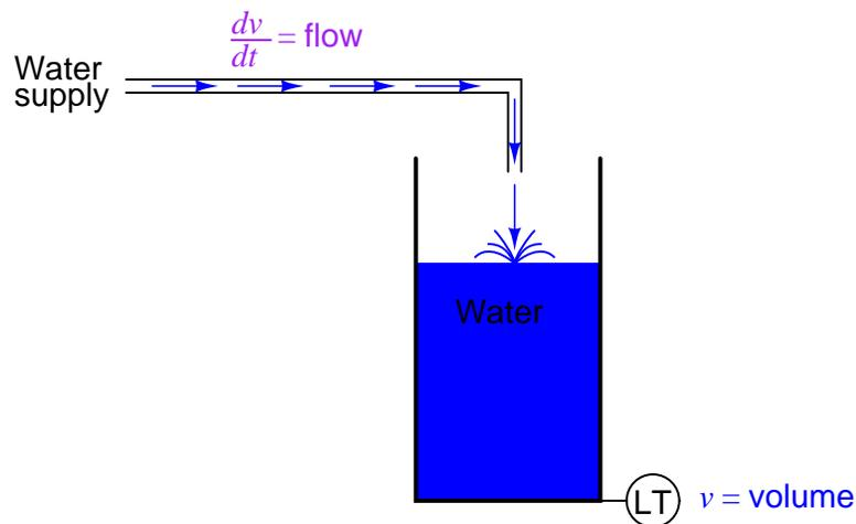
A "Level Transmitter" device mounted on a water storage tank provides a signal directly proportional to water level in the tank, which – if the tank is of constant cross-sectional area throughout its height – directly equates water volume stored. If we were to take this volume signal and differentiate it with respect to time ( $dv/dt$ ), we would obtain a signal proportional to the water *flow rate* through the pipe carrying water to the tank. A differentiator circuit
