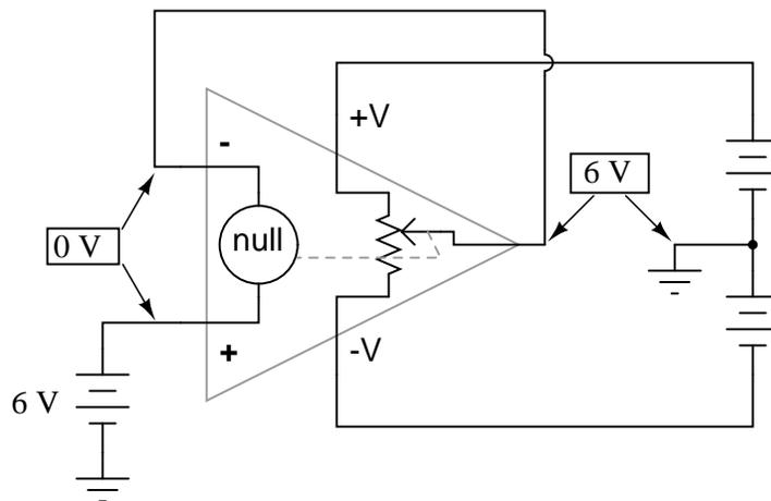
As the "potentiometer" will move to provide an output voltage necessary to satisfy the "null detector" at an "indication" of zero volts, the output voltage becomes equal to the input voltage: in this case, 6 volts. If the input voltage changes at all, the "potentiometer" inside the op-amp will change position to hold the "null detector" in balance (indicating zero volts), resulting in an output voltage approximately equal to the input voltage at all times.
