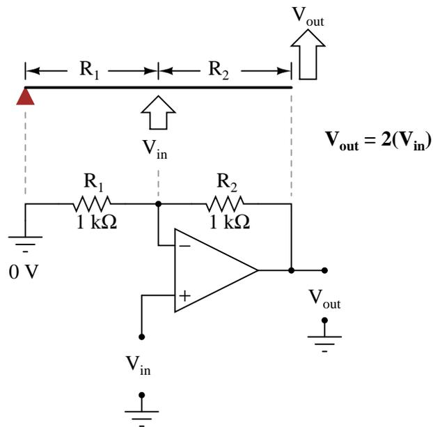
Physicists call this type of lever, with the input force (effort) applied between the fulcrum and output (load), a *third-class* lever. It is characterized by an output displacement (motion) at least as large than the input displacement – a “gain” of at least 1 – and in the same direction. Applying a positive input voltage to this op-amp circuit is analogous to displacing the “input” point on the lever upward:
