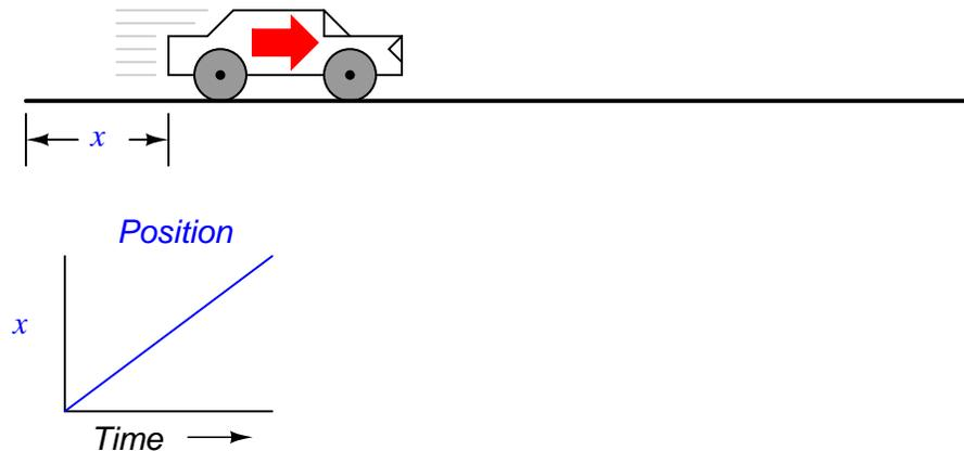
If we were to calculate the *derivative* of the car's position with respect to time (that is, determine the rate-of-change of the car's position with respect to time), we would arrive at a quantity representing the car's velocity. The differentiation function is represented by the fractional notation  $d/d$ , so when differentiating position ( $x$ ) with respect to time ( $t$ ), we denote the result (the derivative) as  $dx/dt$ :
