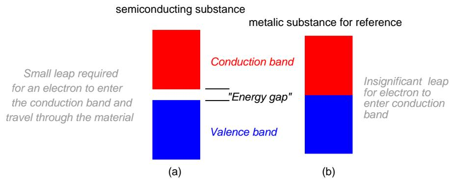
Figure 2.22: *Electron band separation in semiconducting substances, (a) multitudes of semi-conducting close atoms still results in a significant band gap, (b) multitudes of close metal atoms for reference.*
