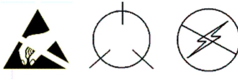
These are some of the more common logos associated with anti-static labels. They are used to inform the user that the contents are static sensitive.
