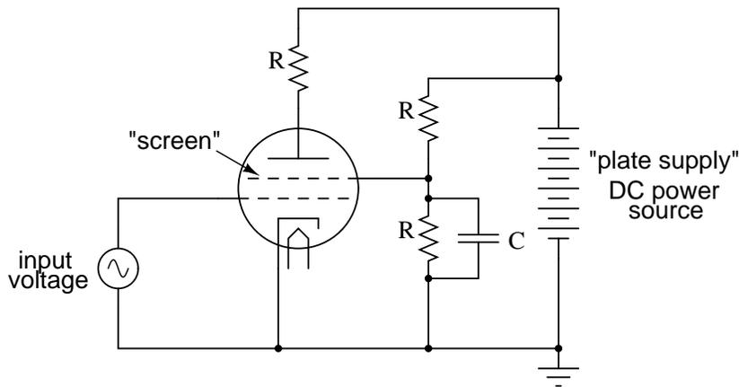
With a constant DC screen voltage, electron flow from cathode to plate became almost exclusively dependent upon grid voltage, meaning the plate voltage could vary over a wide range with little effect on plate current. This made for more stable gains in amplifier circuits, and better linearity for more accurate reproduction of the input signal waveform.
