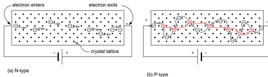
Figure 2.26: (a) *N-type semiconductor with electrons moving left to right through the crystal lattice. (b) P-type semiconductor with holes moving left to right, which corresponds to electrons moving in the opposite direction.*
