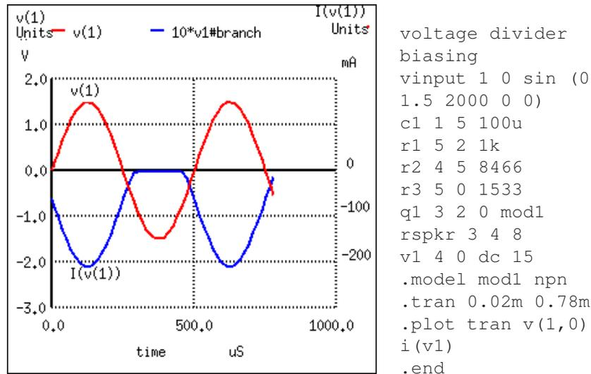
Figure 4.82: SPICE simulation of voltage divider bias.
