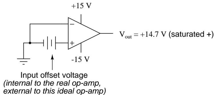
Offset voltage will tend to introduce slight errors in any op-amp circuit. So how do we compensate for it? Unlike common-mode gain, there are usually provisions made by the manufacturer to trim the offset of a packaged op-amp. Usually, two extra terminals on the op-amp package are reserved for connecting an external "trim" potentiometer. These connection points are labeled *offset null* and are used in this general way:
