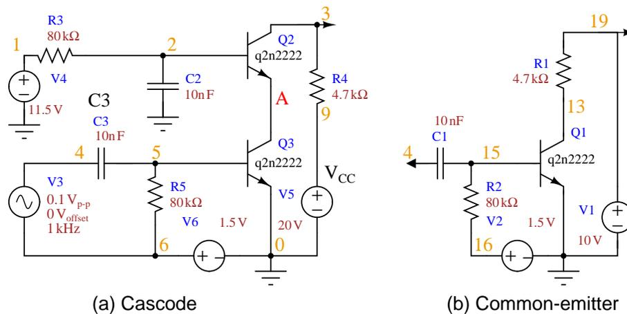
Figure 4.62: SPICE: Cascode and common-emitter for comparison.
