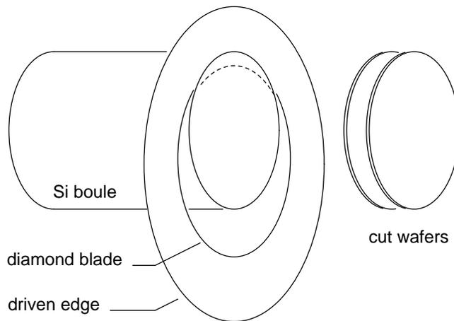
Figure 2.52: Silicon boule is diamond sawed into wafers.
