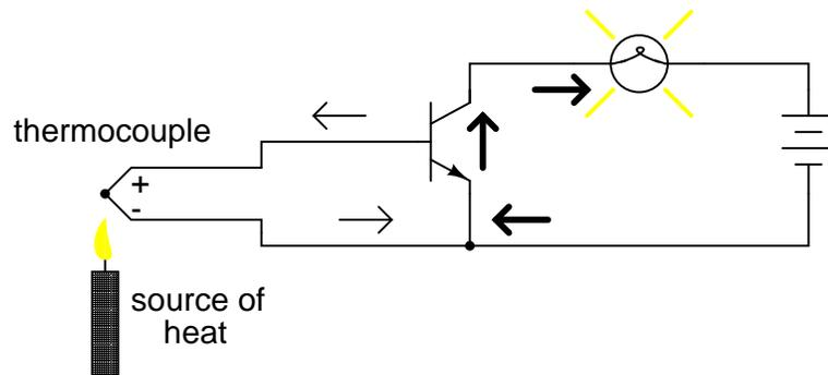
Figure 4.6: A single thermocouple provides less than 40 mV. Many in series could produce in excess of the 0.7 V transistor  $V_{BE}$  to cause base current flow and consequent collector current to the lamp.
