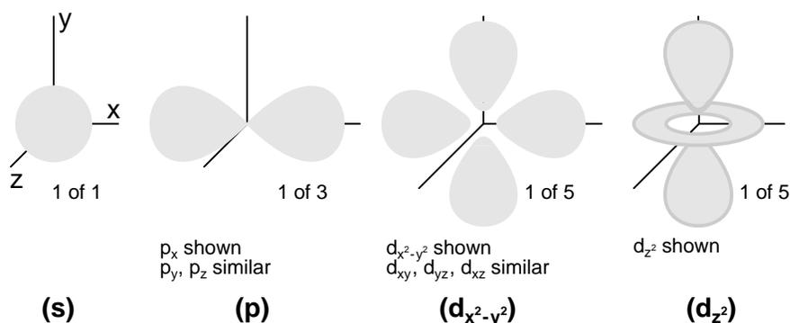
Figure 2.7: Orbitals: (s) Three fold symmetry. (p) Shown:  $p_x$ , one of three possible orientations ( $p_x, p_y, p_z$ ), about their respective axes. (d) Shown:  $d_{x^2-y^2}$  similar to  $d_{xy}, d_{yz}, d_{xz}$ . Shown:  $d_z^2$ . Possible d-orbital orientations: five.
