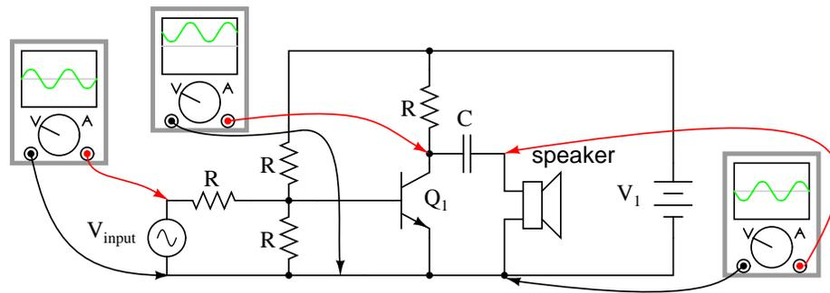
Figure 4.100: *Capacitor coupling isolates DC from the load.*
