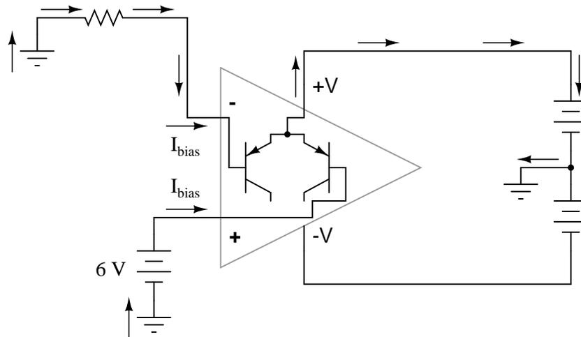
Without a ground reference on the power supply, the bias currents will have no complete path for a circuit, and they will halt. Since bipolar junction transistors are current-controlled devices, this renders the input stage of the op-amp useless as well, as both input transistors will be forced into cutoff by the complete lack of base current.
