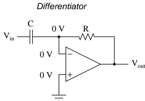
The right-hand side of the capacitor is held to a voltage of 0 volts, due to the "virtual ground" effect. Therefore, current "through" the capacitor is solely due to *change* in the input voltage. A steady input voltage won't cause a current through C, but a *changing* input voltage will.
