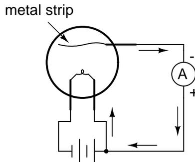
The white-hot filament in Edison's lamp was liberating free electrons into the vacuum of the lamp, those electrons finding their way to the metal strip, through the galvanometer, and back to the filament. His curiosity piqued, Edison then connected a fairly high-voltage battery in the galvanometer circuit to aid the small current:
