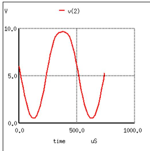
Figure 4.118: *Distortion in large signal common-emitter amplifier.*
