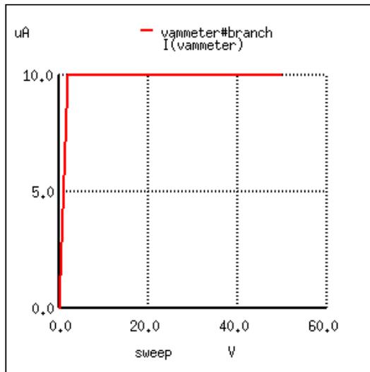
As expected for any transistor, the controlled current holds steady at a regulated value over a wide range of power supply voltages. In this case, that regulated point is  $10 \mu\text{A}$  ( $1.000\text{E-}05$ ). Now let's see what happens when we apply a negative voltage to the gate (with reference to the source) and sweep the power supply over the same range of 0 to 50 volts:
