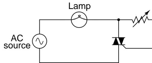
Figure 7.42: This circuit with the gate to  $MT_2$  does function.
