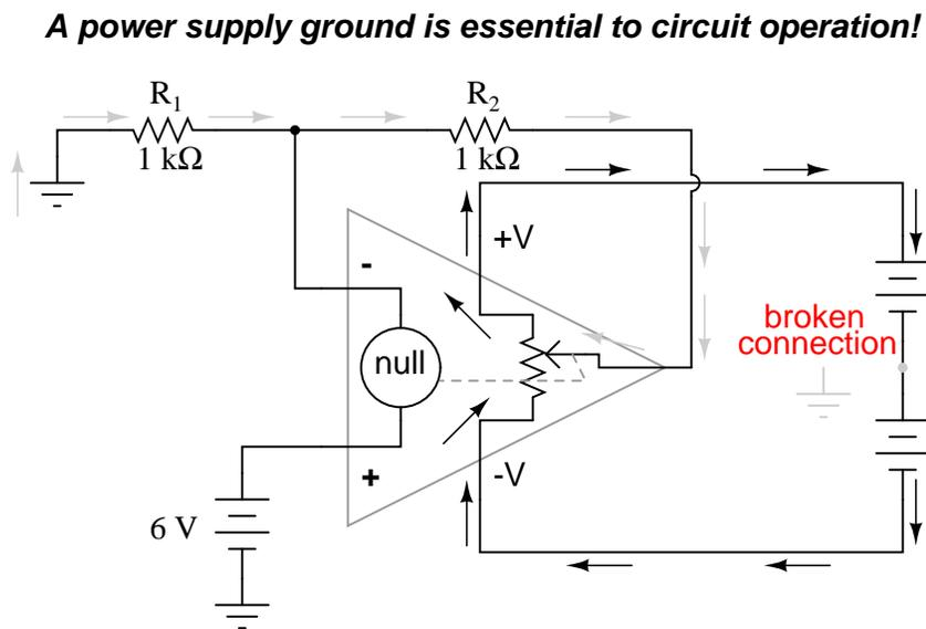
No electrons may flow in or out of the op-amp's output terminal, because the pathway to the power supply is a "dead end." Thus, no electrons flow through the ground connection to the left of  $R_1$ , neither through the feedback loop. This effectively renders the op-amp useless: it can neither sustain current through the feedback loop, nor through a grounded load, since there is no connection from any point of the power supply to ground.
