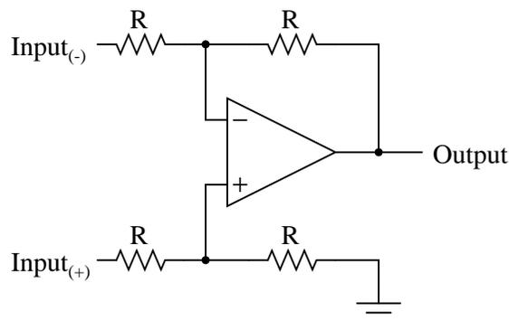
$$\text{Output} = \text{Input}_{(+)} - \text{Input}_{(-)}$$
