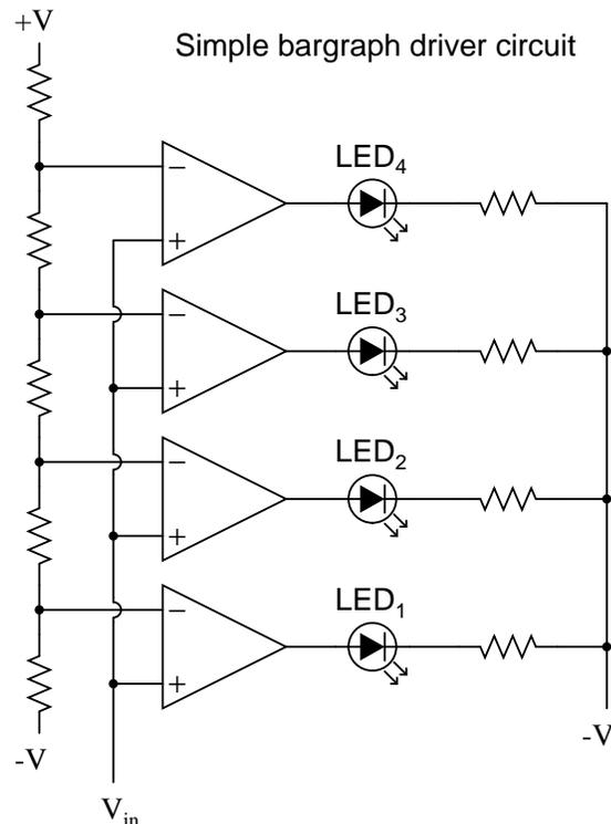
In the circuit shown above, LED<sub>1</sub> would be the first to light up as the input voltage increased in a positive direction. As the input voltage continued to increase, the other LED's would illuminate in succession, until all were lit.
