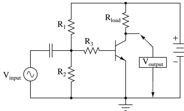
Figure 4.104: *Common-emitter amplifier without feedback.*
