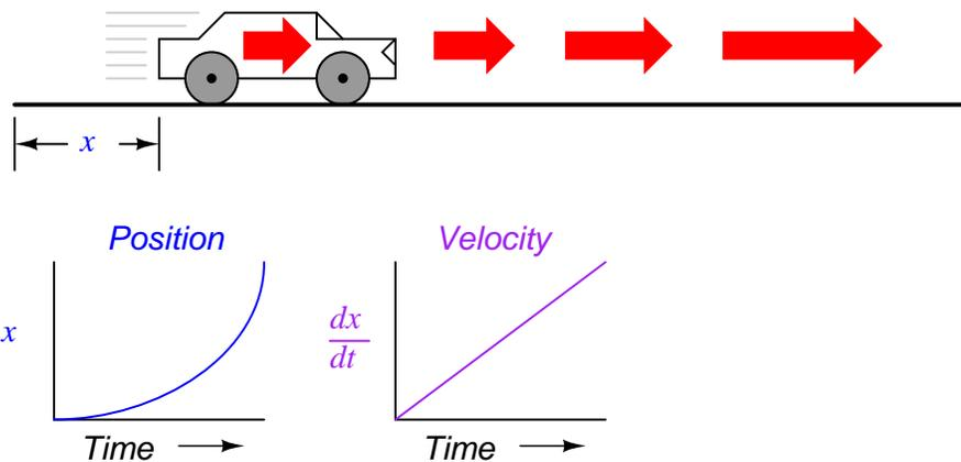
The height of points on the velocity graph correspond to the rates-of-change, or slope, of points at corresponding times on the position graph:
