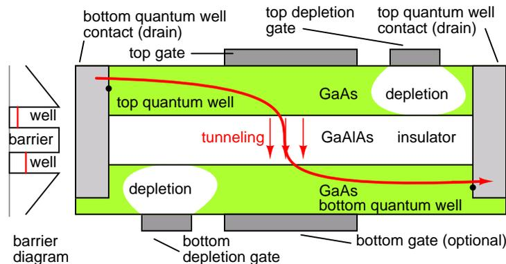
Figure 2.60: *Double-layer tunneling transistor (Deltt) is composed of two electron containing wells separated by a nonconducting barrier. The gate voltages may be adjusted so that the energy and momentum of the electrons in the wells are equal which permits electrons to tunnel through the nonconductive barrier. (The energy levels are shown as unequal in the barrier diagram.)*
