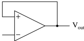
The inverting input remains disconnected from the feedback loop, and is free to receive an external voltage. Let's see what happens if we ground the inverting input:
