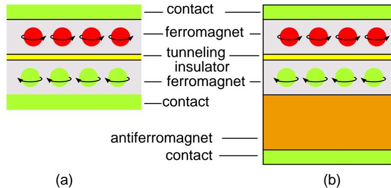
Figure 2.64: (a) *Magnetic tunnel junction (MTJ):* Pair of ferromagnetic layers separated by a thin insulator. The resistance varies with the magnetization polarity of the top layer (b) *Antiferromagnetic bias magnet and pinned bottom ferromagnetic layer* increases resistance sensitivity to changes in polarity of the top ferromagnetic layer. Adapted from [9] Figure 3.
