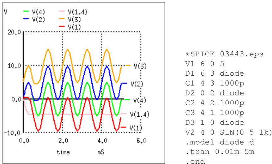
Figure 3.38:  $V(4)$  source voltage 5 V peak used in all clampers.  $V(1)$  clamper output from Figure 3.37 (a).  $V(1,4)$  DC voltage on capacitor in Figure (a).  $V(2)$  clamper output from Figure (b).  $V(3)$  clamper output from Figure (c).
