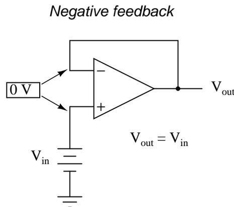
Whether the output is directly fed back to the inverting (-) input or coupled through a set of components, the effect is the same: the extremely high differential voltage gain of the op-amp will be "tamed" and the circuit will respond according to the dictates of the feedback "loop" connecting output to inverting input.
