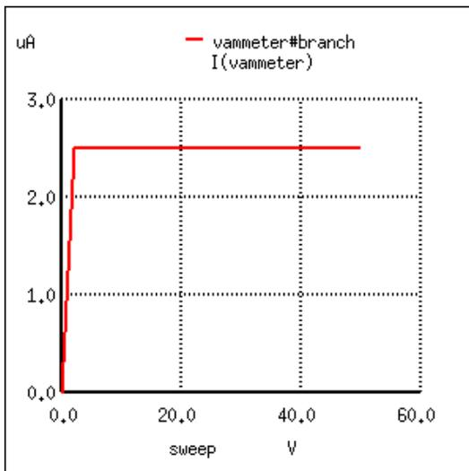
Not surprisingly, the drain current is now regulated at a lower value of  $2.5 \mu\text{A}$  (down from  $10 \mu\text{A}$  with zero input voltage). Now let's apply an input voltage of the other polarity, to *enhance* the IGFET:
