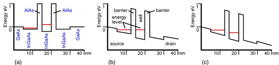
Figure 2.59: *Resonant tunneling diode (RTD): (a) No bias, source and well energy levels not matched, no conduction. (b) Small bias causes matched energy levels (resonance); conduction results. (c) Further bias mismatches energy levels, decreasing conduction.*
