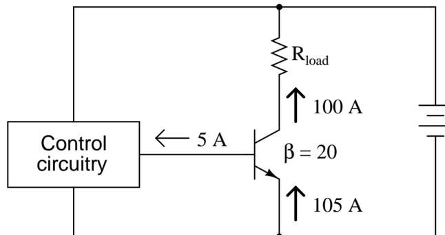
It would be nice from the standpoint of control circuitry to have power transistors with high current gain, so that far less current is needed for control of load current. Of course, we can use Darlington pair transistors to increase the current gain, but this kind of arrangement still requires *far* more controlling current than an equivalent power IGFET:
