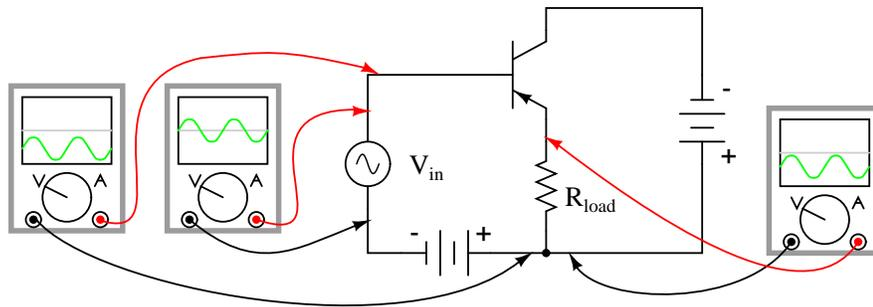
Figure 4.47: PNP version of the common-collector amplifier.
