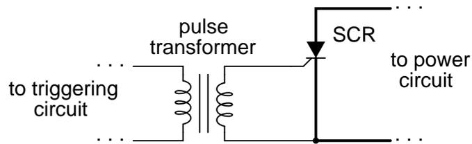
Figure 7.34: Transformer coupling of trigger signal provides isolation.
