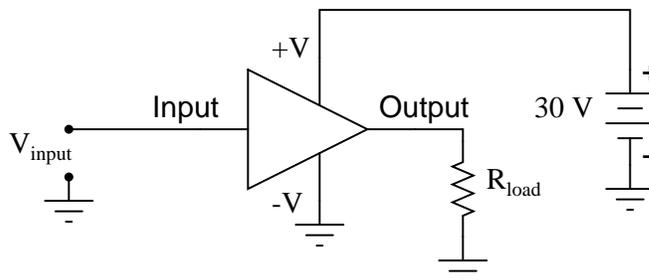
Without having to analyze the actual transistor design of the amplifier, you can readily discern the whole circuit's function: to take an input signal ( $V_{in}$ ), amplify it, and drive a load
