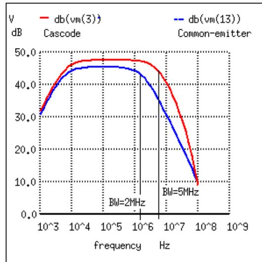
Figure 4.64: Cascode vs common-emitter bandwidth.
