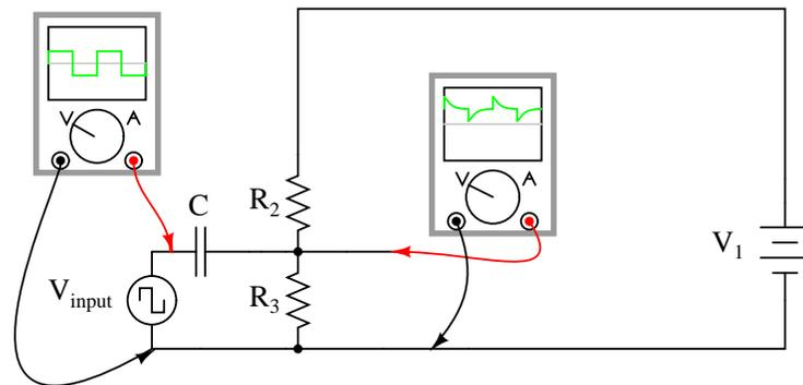
Figure 4.95: *Capacitively coupled low frequency square-wave shows distortion.*
