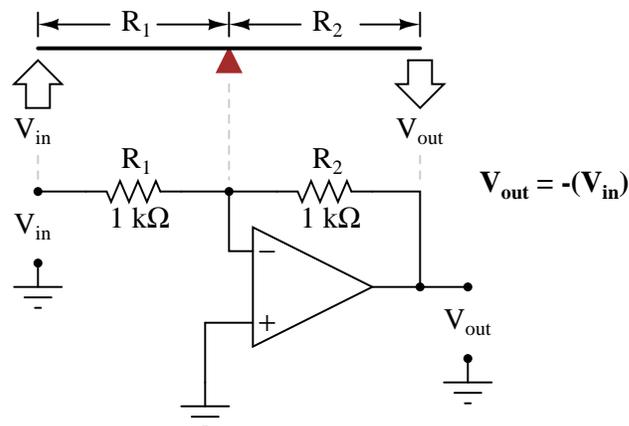
With equal-value resistors (equal-lengths of lever on each side of the fulcrum), the output voltage (displacement) will be equal in magnitude to the input voltage (displacement), but of the opposite polarity (direction). A positive input results in a negative output:
