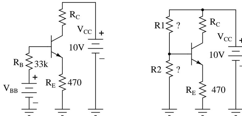
Figure 4.92: *Emitter-bias example converted to voltage divider bias.*
