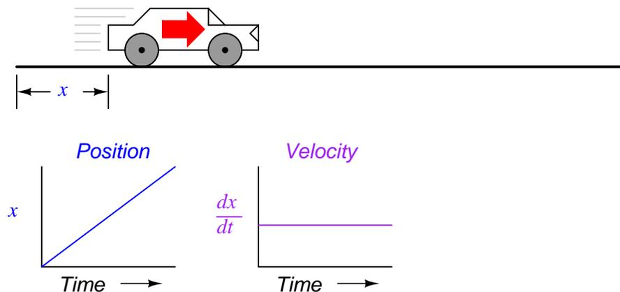
For a linear graph of  $x$  over time, the derivative of position ( $dx/dt$ ), otherwise and more commonly known as *velocity*, will be a flat line, unchanging in value. The derivative of a mathematical function may be graphically understood as its *slope* when plotted on a graph,
