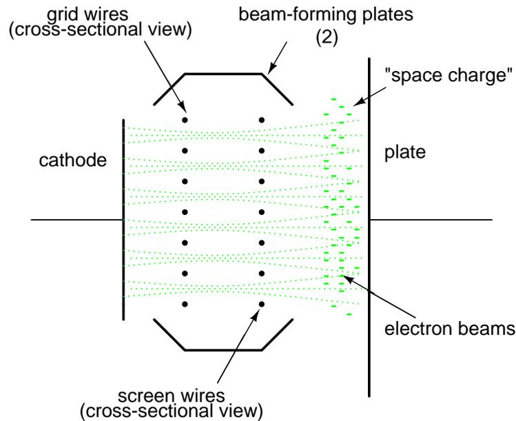
This resulted in lower screen current (and more plate current!) than an ordinary tetrode tube, with little added expense to the construction of the tube.
