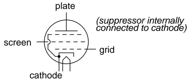
The suppressor's job was to repel any secondarily emitted electrons back to the plate: a structural equivalent of the beam power tube's space charge. This, of course, increased plate current and decreased screen current, resulting in better gain and overall performance. In some instances it allowed for greater operating plate voltage as well.
