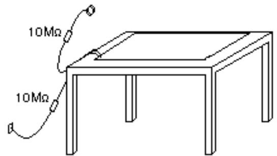
Incorrectly grounded station, the wrist strap is connected to the table surface, in the event of ESD in the wrist strap it will also raise the table's potential. This is better than no protection.
