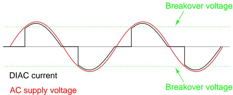
Figure 7.18: DIAC waveforms
