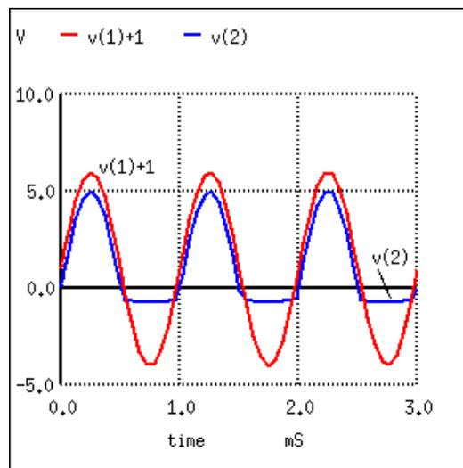
Figure 3.31:  $V(1)+1$  is actually  $V(1)$ , a 10 V<sub>ptp</sub> sinewave, offset by 1 V for display clarity.  $V(2)$  output is clipped at  $-0.7$  V, by diode D1.
