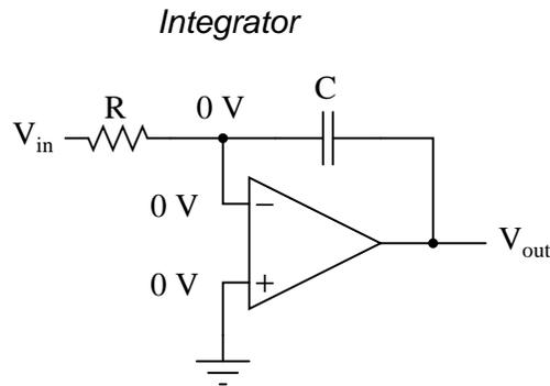
As before, the negative feedback of the op-amp ensures that the inverting input will be held at 0 volts (the virtual ground). If the input voltage is exactly 0 volts, there will be no current through the resistor, therefore no charging of the capacitor, and therefore the output voltage will not change. We cannot guarantee what voltage will be at the output with respect to ground in this condition, but we can say that the output voltage *will be constant*.
