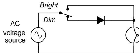
Figure 3.15: *Half-wave rectifier application: Two level lamp dimmer.*
