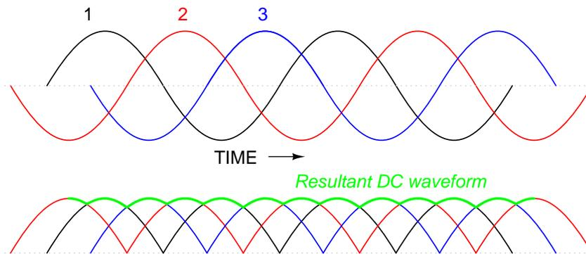
Figure 3.26: Three-phase AC and 3-phase full-wave rectifier output.
