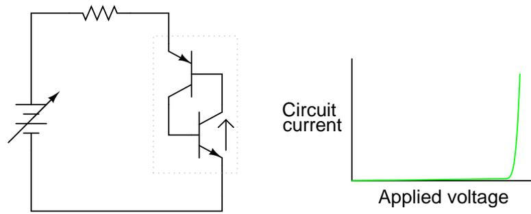
Figure 7.11: *More voltage applied; lower transistor breaks down*
