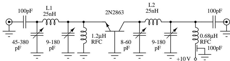
Figure 9.19: Class C common-base 750 mW RF power amplifier.  $L1 = \#10$  Cu wire  $1/2$  turn,  $5/8$  in. ID by  $3/4$  in. high.  $L2 = \#14$  tinned Cu wire  $1 1/2$  turns,  $1/2$  in. ID by  $1/3$  in. spacing. After Texas Instruments [5]
