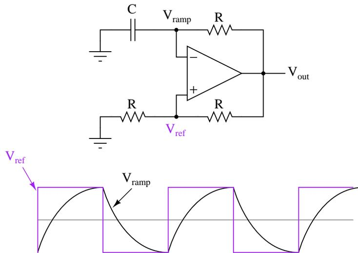
$V_{out}$  is a square wave just like  $V_{ref}$ , only taller
