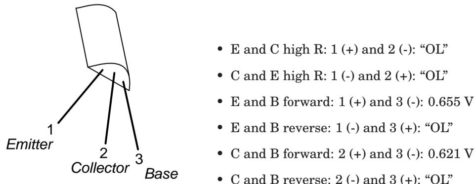
Figure 4.10: BJT terminals identified by  $\Omega$ -meter.
