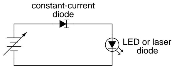
Figure 3.85: Constant current diode application: driving laser diode.
