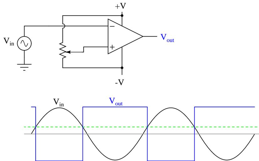
Adjustments to the potentiometer setting would change the reference voltage applied to the noninverting (+) input, which would change the points at which the sine wave would cross, changing the on/off times, or *duty cycle* of the square wave:
