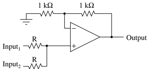
$$\text{Output} = \text{Input}_1 + \text{Input}_2$$
