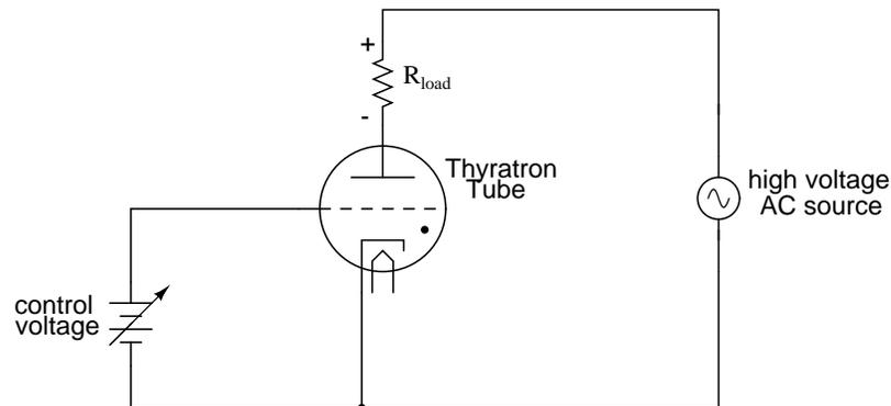
It should be noted that the schematic shown above is greatly simplified for most purposes and thyatron tube designs. Some thyratrons, for instance, required that the grid voltage switch polarity between their "on" and "off" states in order to properly work. Also, some thyratrons had more than one grid!
