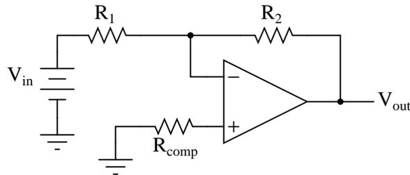
$$R_{\text{comp}} = R_1 \parallel R_2$$
