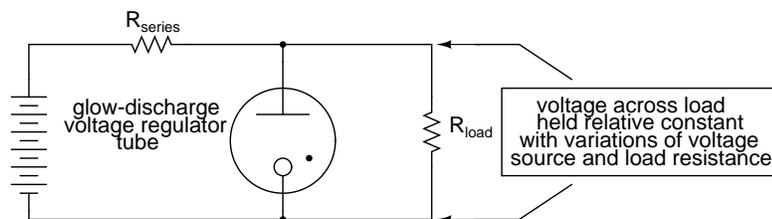
Please take note of the black dot found in the tube symbol shown above (and in the neon lamp symbol shown before that). That marker indicates the tube is gas-filled. It is a common marker used in all gas-filled tube symbols.
