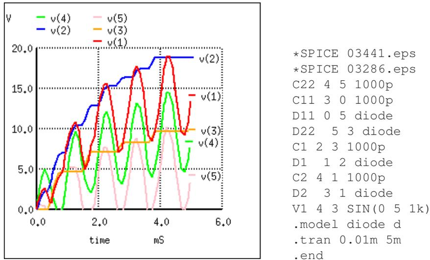
Figure 3.47: Voltage quadrupler: DC voltage available at  $v(3)$  and  $v(2)$ . Intermediate waveforms: Clampers:  $v(5)$ ,  $v(4)$ ,  $v(1)$ .
