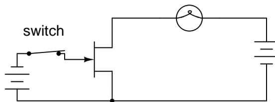
Note that there is no current going through the gate. As a reverse-biased PN junction, it firmly opposes the flow of any electrons through it. As a voltage-controlled device, the JFET requires negligible input current. This is an advantageous trait of the JFET over the bipolar transistor: there is virtually zero power required of the controlling signal.
