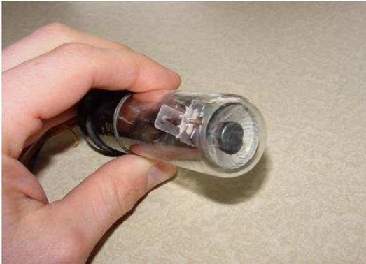
Normally, only the end of the tube would protrude from a hole in an instrument panel, so the user could view the circular, fluorescent screen.
