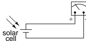
Figure 4.22: *High intensity light directly drives light meter.*
