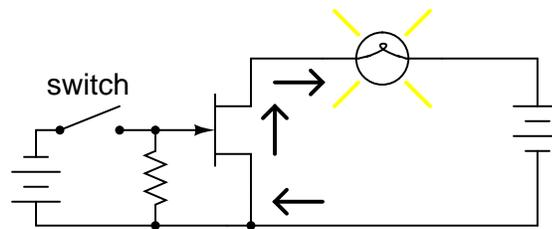
This resistor's value is not very important. The capacitance of the JFET's gate-source junction is very small, and so even a rather high-value bleed resistor creates a fast RC time constant, allowing the transistor to resume conduction with little delay once the switch is opened.
