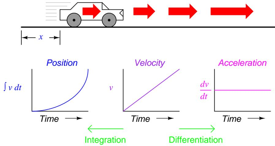
If we had an accelerometer attached to the car, generating a signal proportional to the rate of acceleration or deceleration, we could (hypothetically) obtain a velocity signal with one step of integration, and a position signal with a second step of integration:
