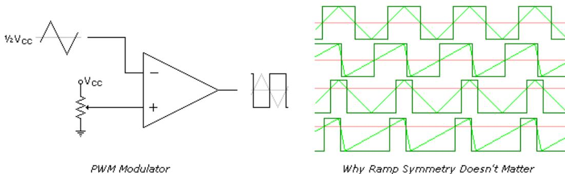
If there isn't any computation involved PWM can be fast. The limiting factor is the comparators frequency response. This may not be an issue since quite a few of the uses are fairly low speed. Some microcontrollers have PWM built in, and can record or create signals on demand.
