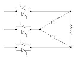
Figure 7.1. Six SCR in-line control
