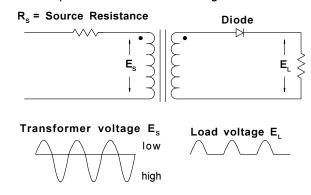
Figure 8.1. Transformer saturation due to secondary DC current
