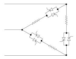
Figure 7.2. Six SCR inside-delta control
