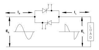
Figure 6.1. Phase angle control at 50% power
