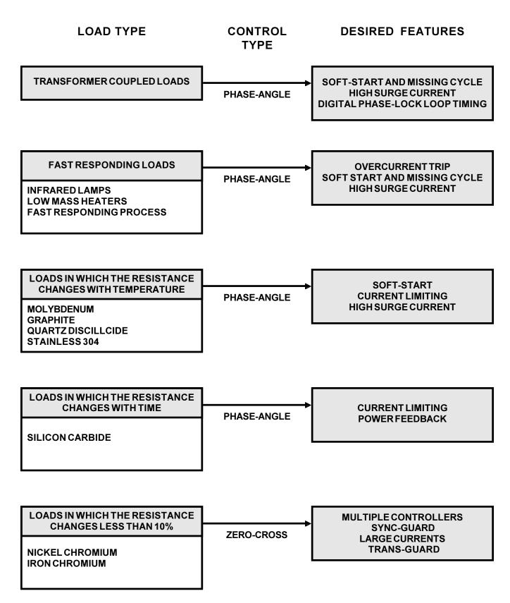
Figure 10.1 SCR Controller Selection Guide
