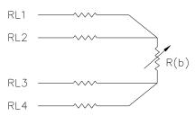
The 4-wire circuit is a true 4-wire bridge, which works by using wires 1 & 4 to power the circuit and wires 2 & 3 to read. This true bridge method will compensate for any differences in lead wire resistances.
