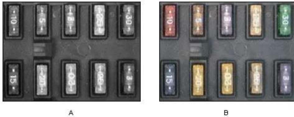
**FIGURE 18: COLOR MATCHING AUTOMOBILE FUSES**
