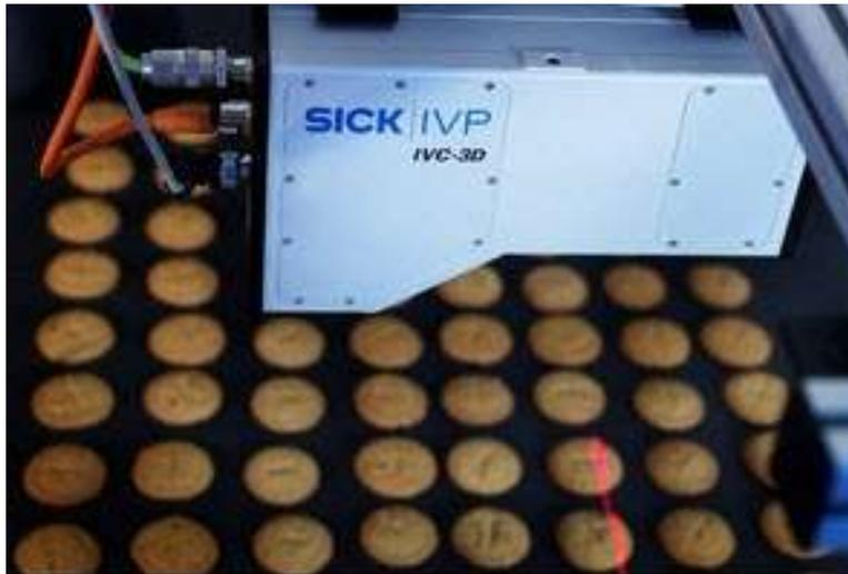
**FIGURE 20: INSPECTION OF COOKIES MOVING RAPIDLY DOWN CONVEYOR LINE**
