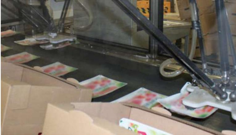
**FIGURE 29: PACKAGING INSPECTION USING MV TO INSURE AIR-TIGHT SEAL**
