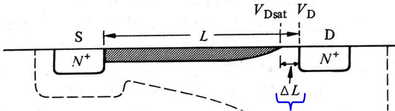
High electric fields in this region act similarly to the collector-base junction in a BJT in active mode, “stripping” or “collecting” carriers from the channel.
