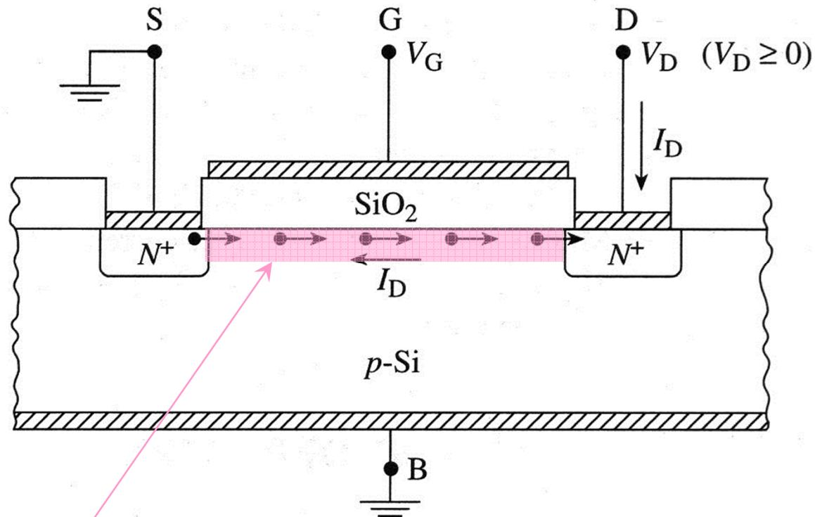
Control by the Gate voltage is achieved by modulating the conductivity of the semiconductor region just below the gate. This region is known as the channel
