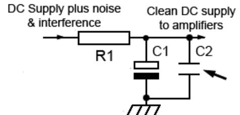
Electrolytic capacitor C1 decouples low frequencies & polyester capacitor C2 gives extra decoupling at HF
