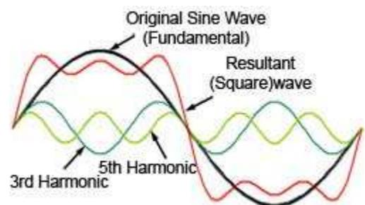
Fig. 3.4.6 The Effect of Adding In-phase Odd Harmonics
