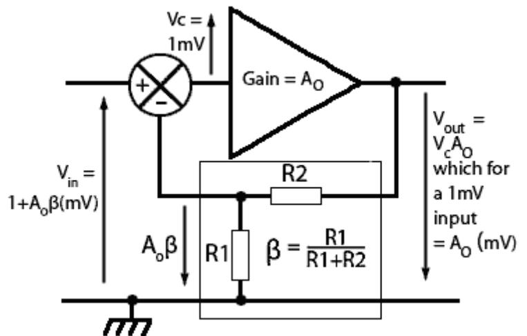
Fig. 3.1.2 Closed Loop Mode
