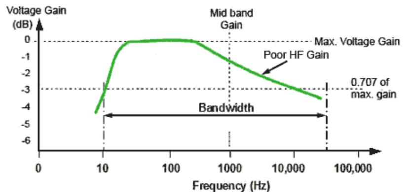
Fig. 3.4.4 Insufficient HF gain.
