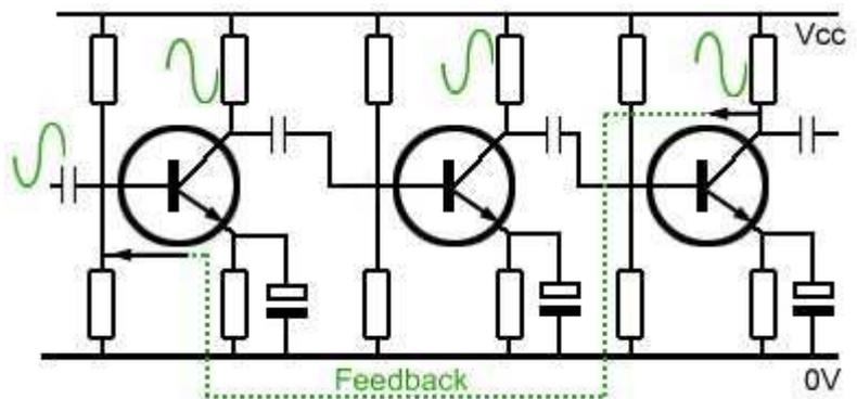
**Fig. 3.2.5 Current Derived, Parallel Fed NFB**
