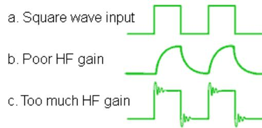
Fig. 3.4.5 Frequency distortion
