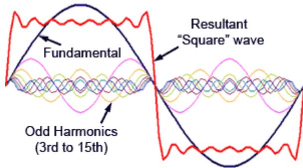
Fig. 3.4.2 Adding odd harmonics to a sine wave.
