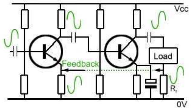
**Fig. 3.2.4 Voltage Derived, Parallel Fed NFB**
