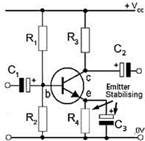
Fig 3.2.1 Emitter Stabilising Components.
