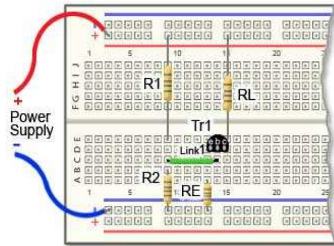
Fig. 2.1.2 Fitting the DC components.
