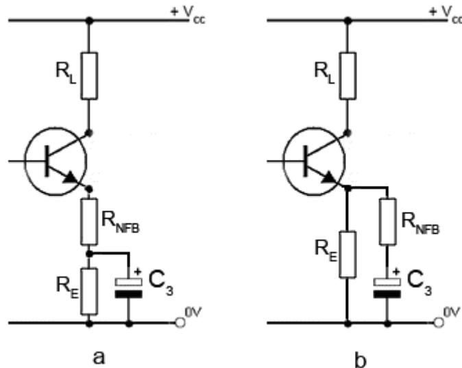
Fig. 2.4.1 Two methods of applying NFB
