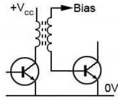
Fig. 2.5.3 Transformer Coupling
