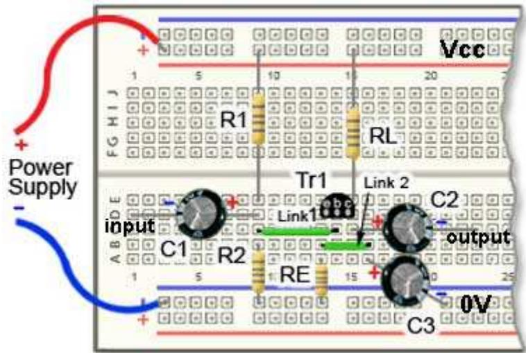
Fig. 2.2.2 Fitting the AC components.
