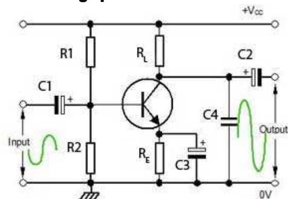
Fig. 2.0.1. Common Emitter Amplifier
