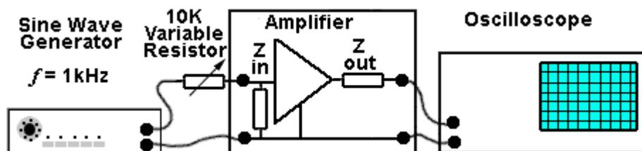
Fig. 2.3.3 Measuring the Amplifier Bandwidth
