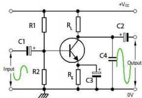
Fig. 2.2.1. Common Emitter Amplifier
