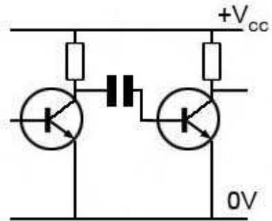
Fig. 2.5.2 Capacitor Coupling
