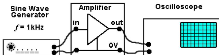
**Fig. 2.3.1 Measuring the Amplifier Gain**
