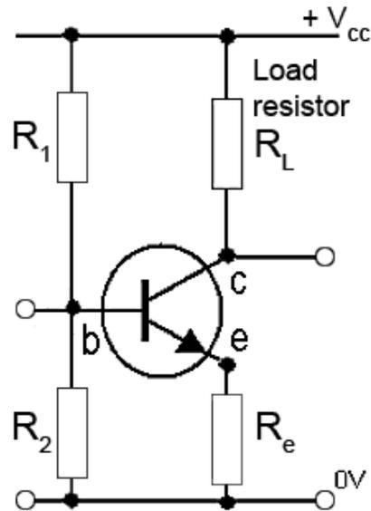
**Fig. 2.1.1 Amplifier DC components**
