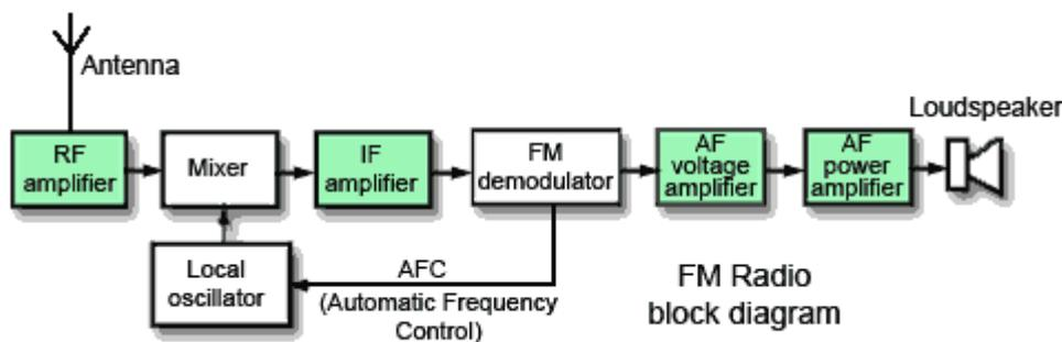
Fig. 1.0.3 FM Radio using AF, IF and RF amplifiers.
