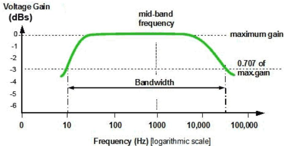
**Fig 1.3.3 Audio Voltage Response Curve**
