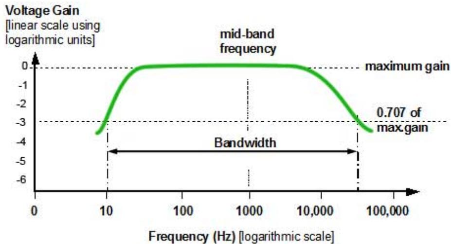
Fig. 1.1.1a Response curve for an audio amplifier
