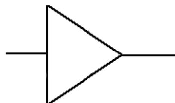
Fig 1.0.1 Amplifier general symbol, used in system diagrams
