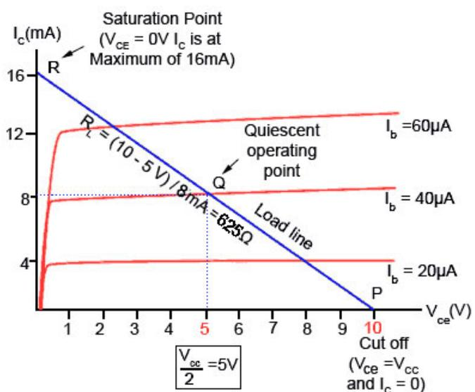
Fig. 1.2.4 Output Characteristics and Load Line
