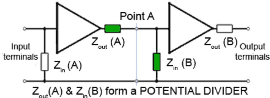
**Fig. 1.1.3 Potential divider effect of amplifiers in Cascade**
