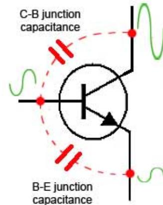
Fig. 1.4.2 Junction Capacitance.
