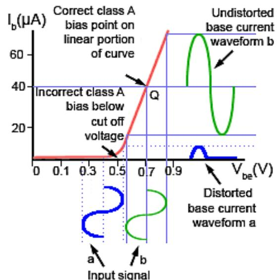
Fig. 1.2.2 Input Characteristics.
