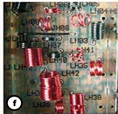
f Air Cored inductors in a TV tuner working at UHF may have very few turns
