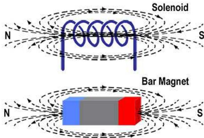
**Fig. 3.1.5 Magnetic Field Around a Solenoid and a Bar Magnet.**
