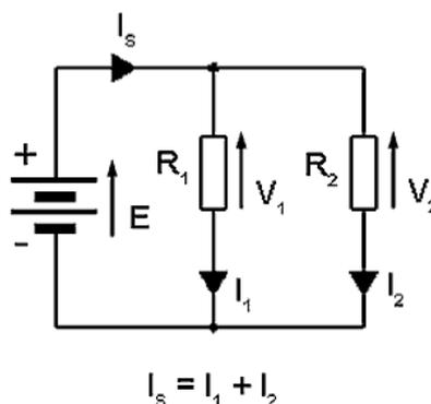
**Fig.4.0.1 A Simple Series Circuit**    **Fig.4.0.2 A Simple Parallel Circuit**
