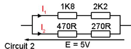
3. Calculate the value of  $I_2$  in Circuit 2
