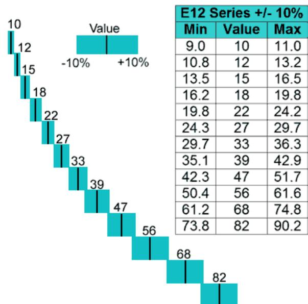
Fig. 2.2.1 E12 Series of Overlapping Tolerances
