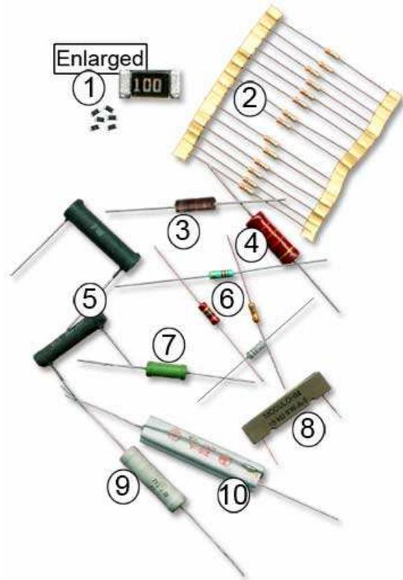
**Fig 2.0.2 Fixed Resistor Types**
