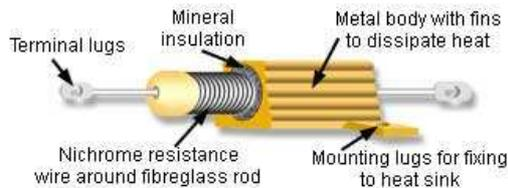
For this reason high power wirewound resistors may be housed in a finned metal case that can be bolted to a metal chassis to dissipate the heat generated as effectively as possible. With all types of wirewound resistor, fire protection is important and flame proof cases or coatings are vital. Lead-out wires are normally welded rather than soldered to the resistor.
