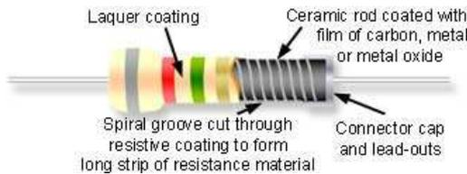
These resistors are made from small rods of ceramic coated with metal such as a nickel alloy or a metal oxide such as tin oxide. The value of resistance is controlled firstly by the thickness of the coating layer; the thicker the layer, the lower the value of resistance.
