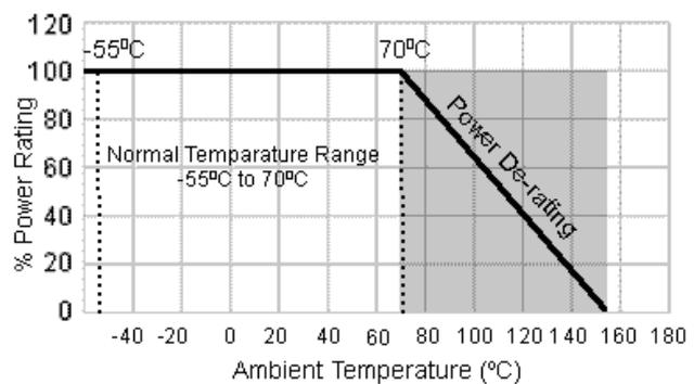
**Fig. 2.4.1 Power De-rating Curve**
