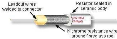
Wirewound resistors are very variable in construction and physical appearance. Their resistive elements are commonly lengths of wire, usually an alloy such as Nichrome (Nickel/Chromium) or Manganin (Copper/Nickel/Manganese) wrapped around a ceramic or glass fibre rod or tube and coated in an insulating flameproof cement film. They are normally available in quite low values of resistance (single ohms to a few Kilohms) but can dissipate large amounts of power. In use they may get very hot.
