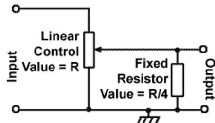
Fig. 2.6.2 Converting a Linear Control to Logarithmic
