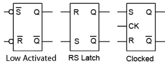
Fig. 5.2.8 SR Flip-flop Circuit Symbols
