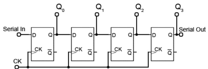
Fig. 5.7.4 Serial In/Parallel Out (SIPO) Shift Register
