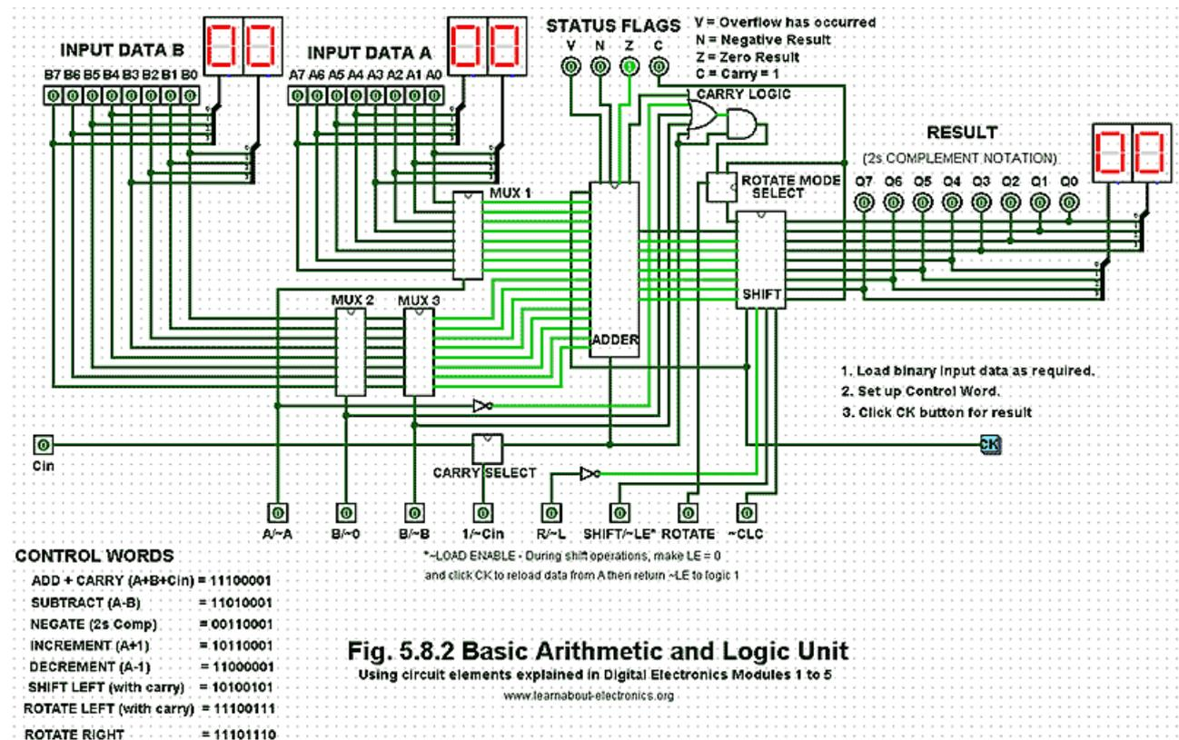
Fig. 5.8.2 Basic Arithmetic and Logic Unit – Logisim Simulation
