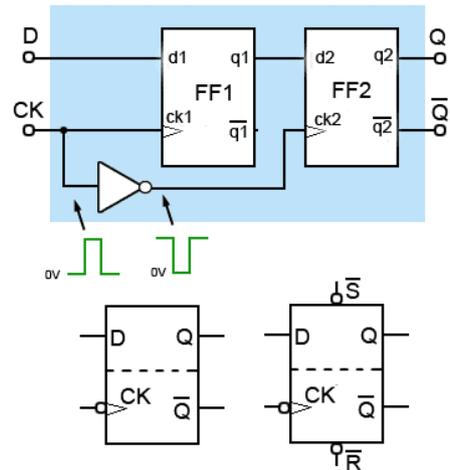
Fig. 5.3.6 The D Type Master Slave Flip-flop
