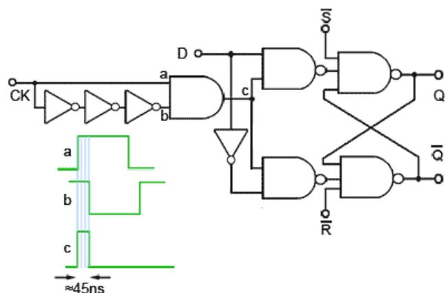
Fig. 5.3.3 Edge Triggered D Type Flip-Flop with Set and Reset
