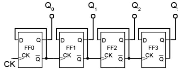
Fig. 5.6.1 Four-bit Asynchronous Up Counter
