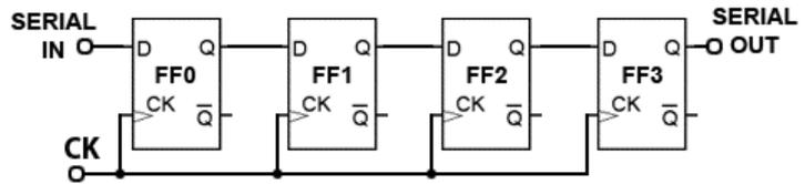
Fig. 5.7.2 Serial In/Serial Out (SISO) Shift Register
