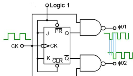
Fig. 5.1.5 Two-Phase Clock Circuit
