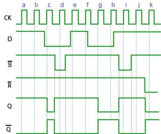
Fig. 5.3.5 Positive Edge Triggered D Type Timing Diagram
