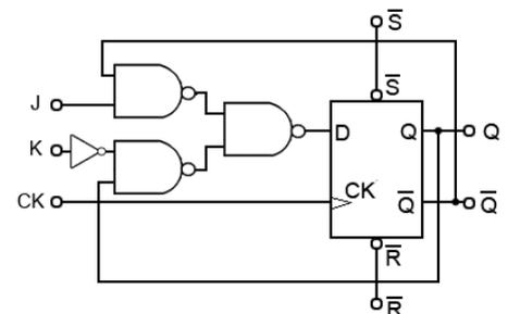
Fig 5.4.5 JK Flip-flop Using a Positive Edge Triggered D Type
