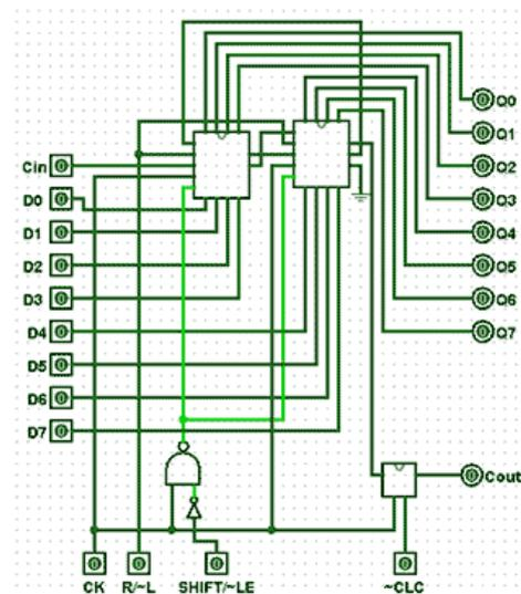
Fig. 5.8.6 The ALU Shift Register Component
