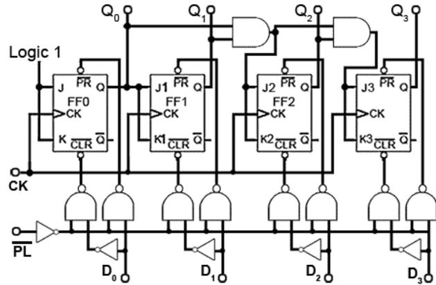
Fig. 5.6.14 Asynchronous Parallel Load
