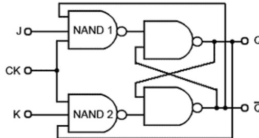
Fig.5.4.1 Basic JK Flip-flop Circuit
