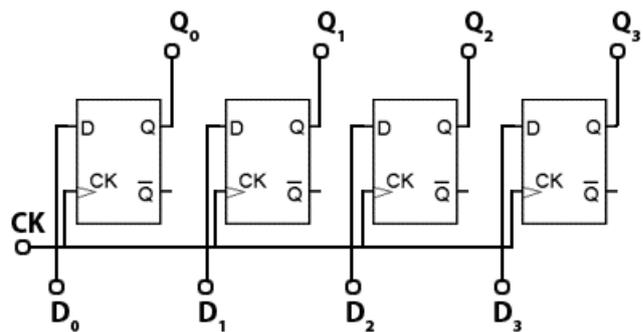
Fig. 5.7.1 Parallel In/Parallel Out (PIPO) Register
