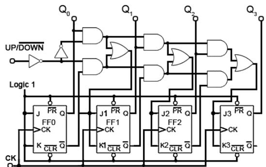
Fig. 5.6.10 Four-bit Synchronous Up/Down Counter
