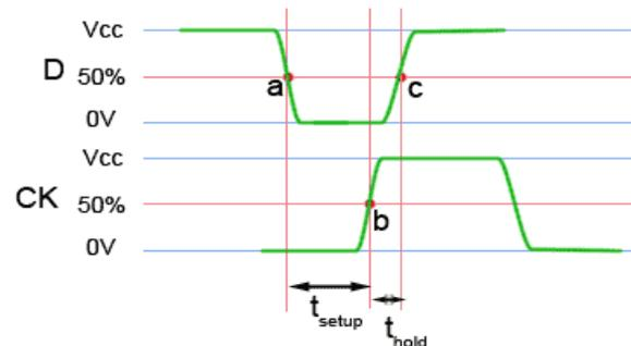
Fig. 5.3.9 Clocked Logic Set Up and Hold Times
