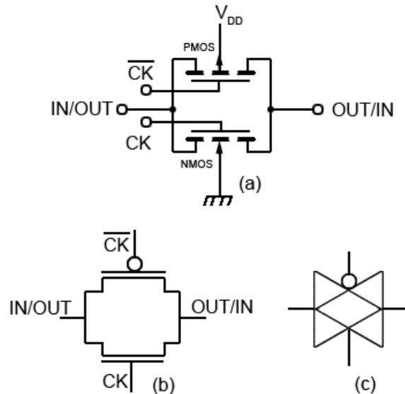
Fig. 5.5.1 The CMOS Transmission Gate
