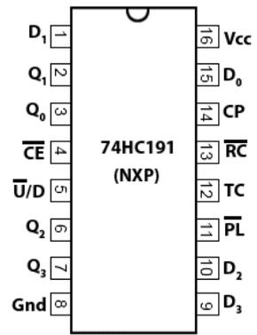
Fig. 5.6.16 74HC191 Pinout
