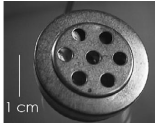
FIGURE 26.6 A crystal microphone 'insert', intended for installing inside a protective case. The crystal is shielded from stray magnetic fields by an aluminium screen. This should be connected to the 0 V line of the amplifier.
