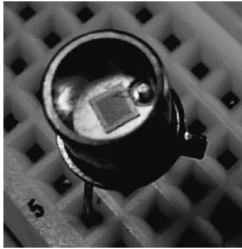
FIGURE 2.3 The can of this photodiode has a lens top. The diode is visible through this as a square chip of silicon.
