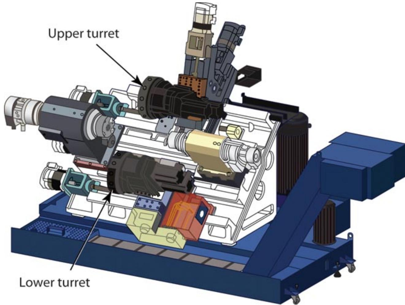
A twin turret machine can move both turrets independently for machining.
