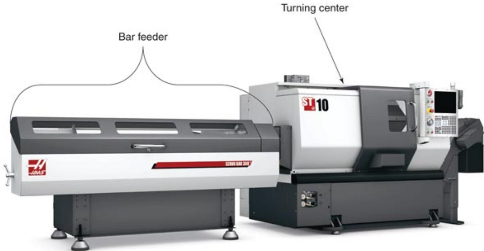
A CNC turning center equipped with an automatic bar feeder.
