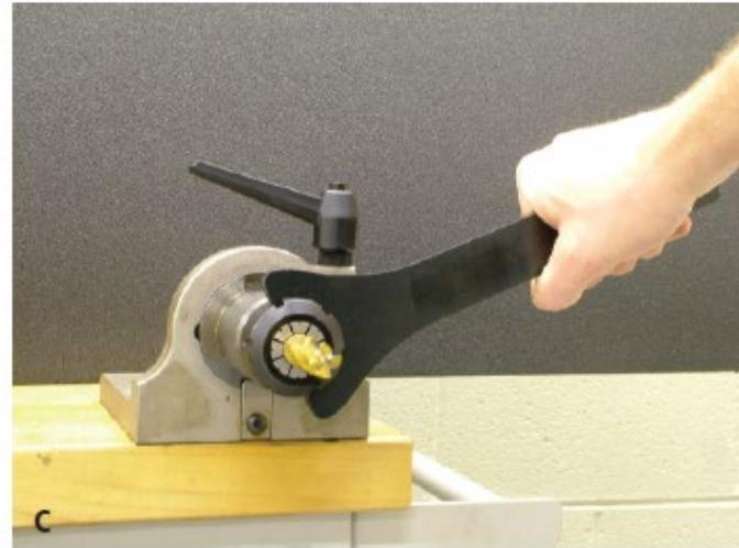
(A) The groove on an ER collet snaps into a retaining ring in the threaded cap and the cap is then threaded into the collet chuck. (B) DA collets slip into the chuck and then the cap is threaded onto the chuck. (C) The toolholder is then mounted in a bench-top clamping device, the tool is inserted in the collet, and the cap is tightened.
