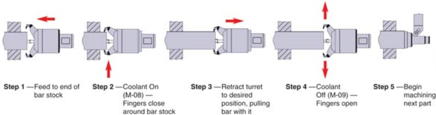
This coolant-actuated bar puller's jaws grip the stock using the hydraulic pressure of the machine's coolant system.
