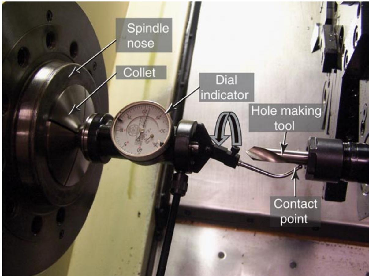
A holeworking tool being swept with a spindle-mounted indicator to find alignment with the spindle axis.
