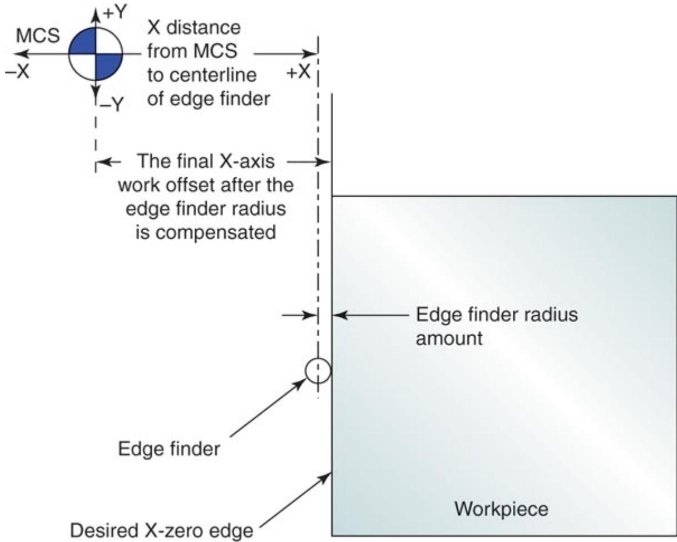
Left-edge workpiece X-zero work offset
