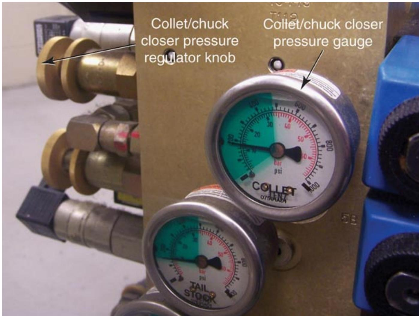
A picture of a turning center hydraulic regulator and gauge for adjusting collet or chuck clamping pressure.
