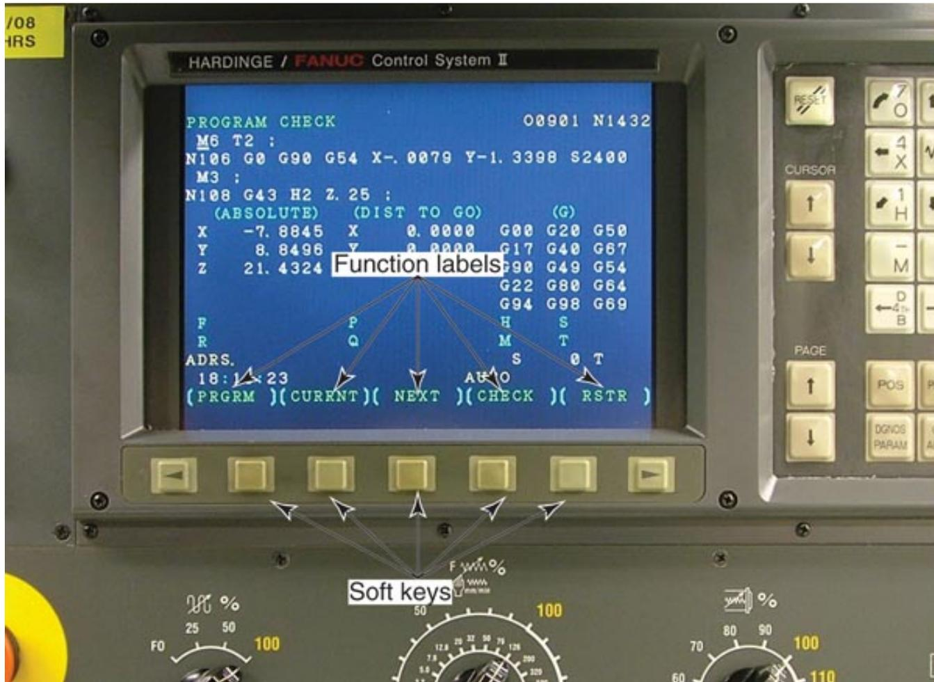
Soft keys are used on some machines. These keys are universal and can be used for different functions according to their on-screen label.
