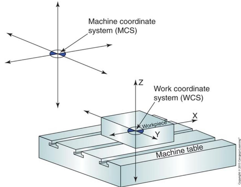
The relationship of the machine coordinate system (MCS) to the work coordinate system (WCS).
