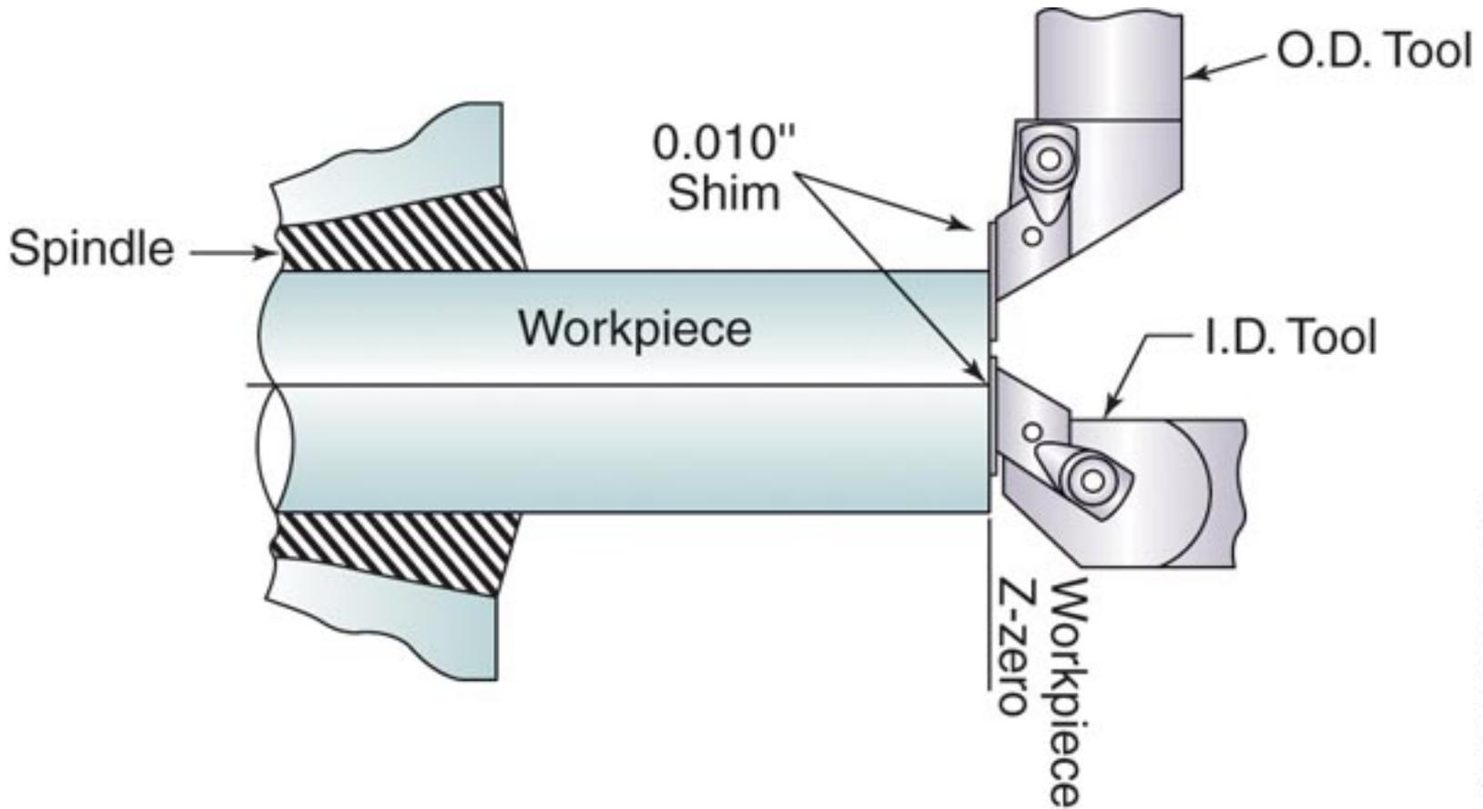
Method for setting tools off the part face of Z-zero with a 0.010"-thick feeler gage. While in this position the tool's position can be set as positive 0.010" in the Z-axis.
