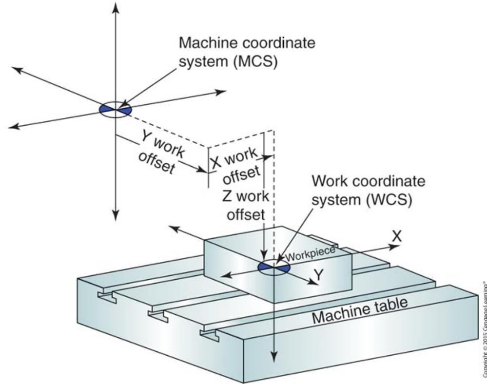
Workpiece offset, or workshift, is the distance from the MCS origin to the desired location of the WCS origin.
