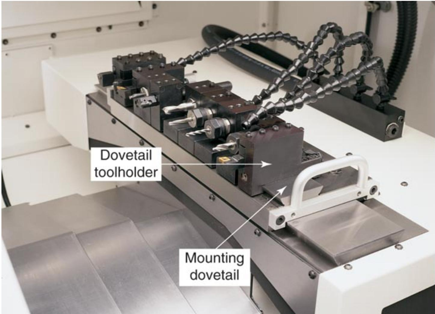
A dovetail mounting system used on a gang tool machine.
