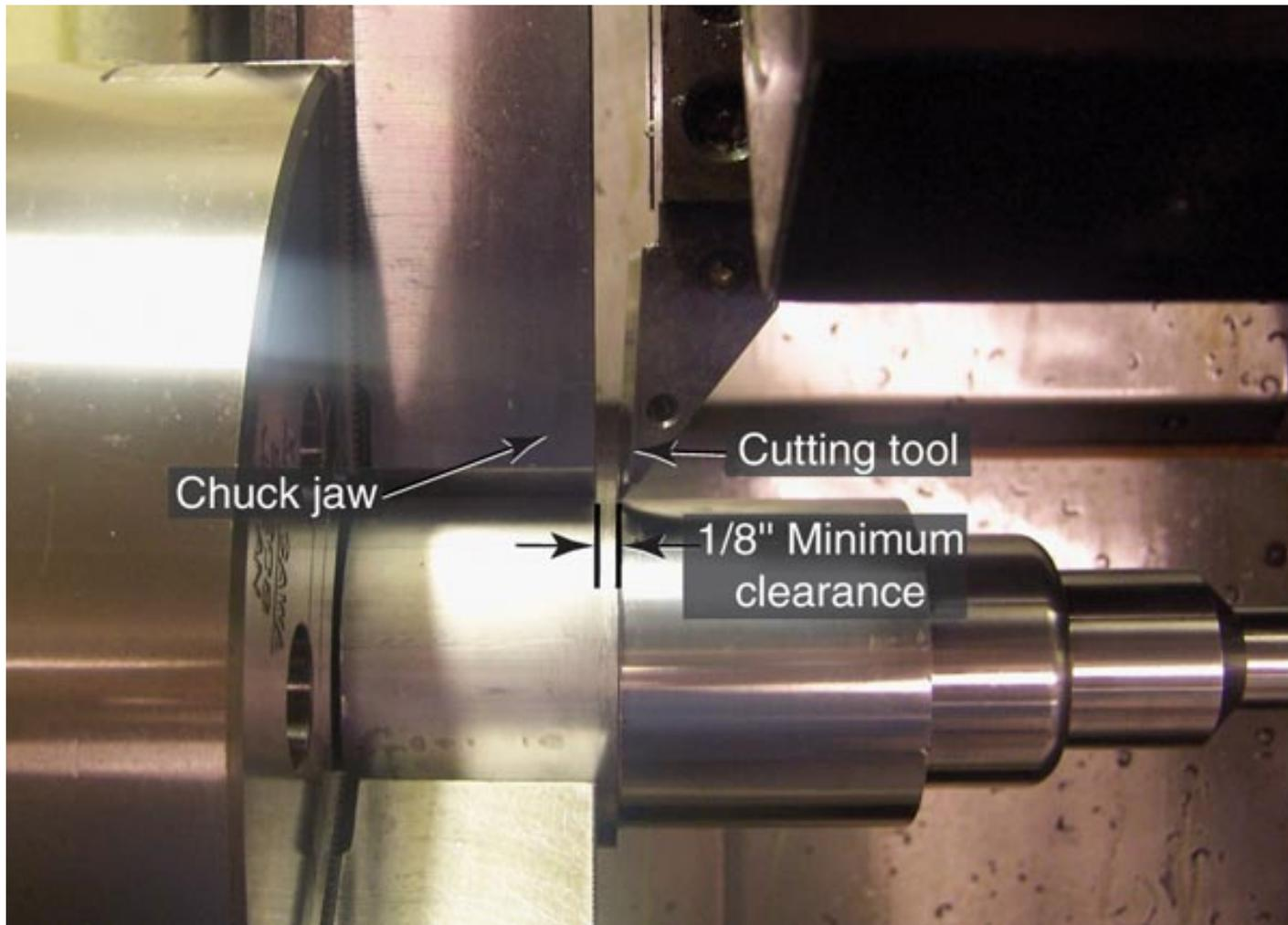
A minimum of 1/8" clearance should be maintained between the cutting tool and the workholding device.
