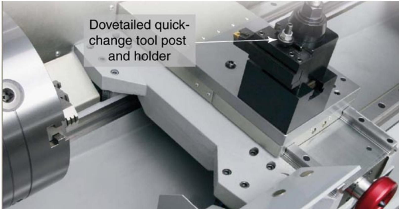
Quick-change toolholders used on a CNC lathe.
