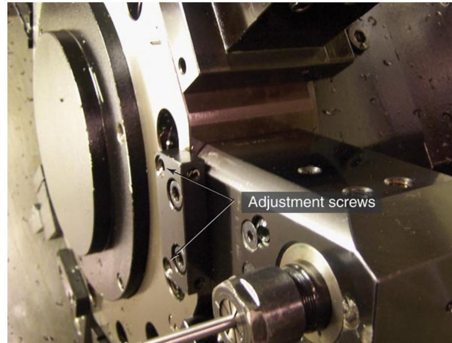
Adjustment screws for squaring a holmaking tool holder.
