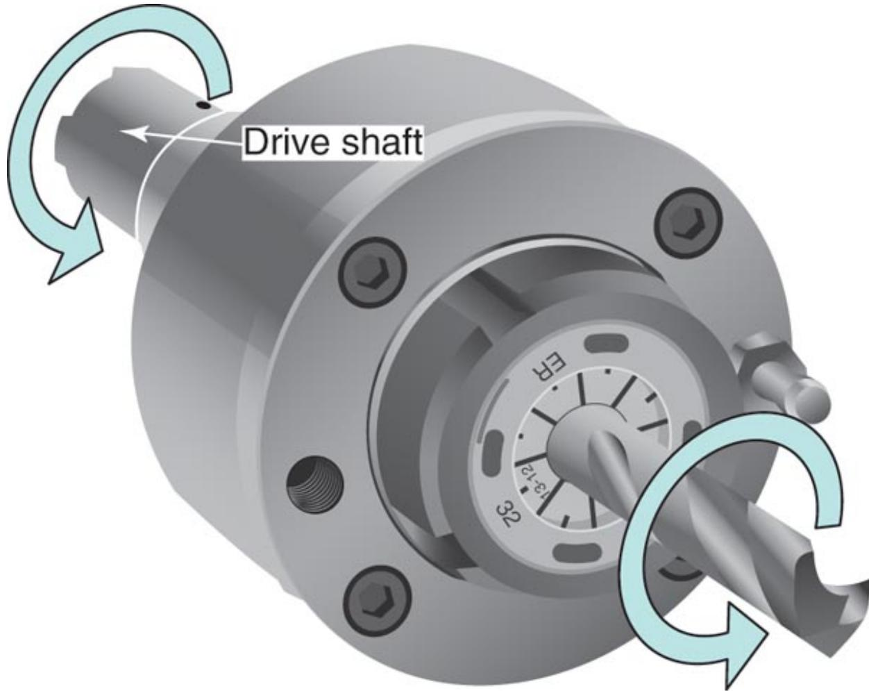
An end-working live tooling attachment for milling and performing holemaking operations on the face of a part.
