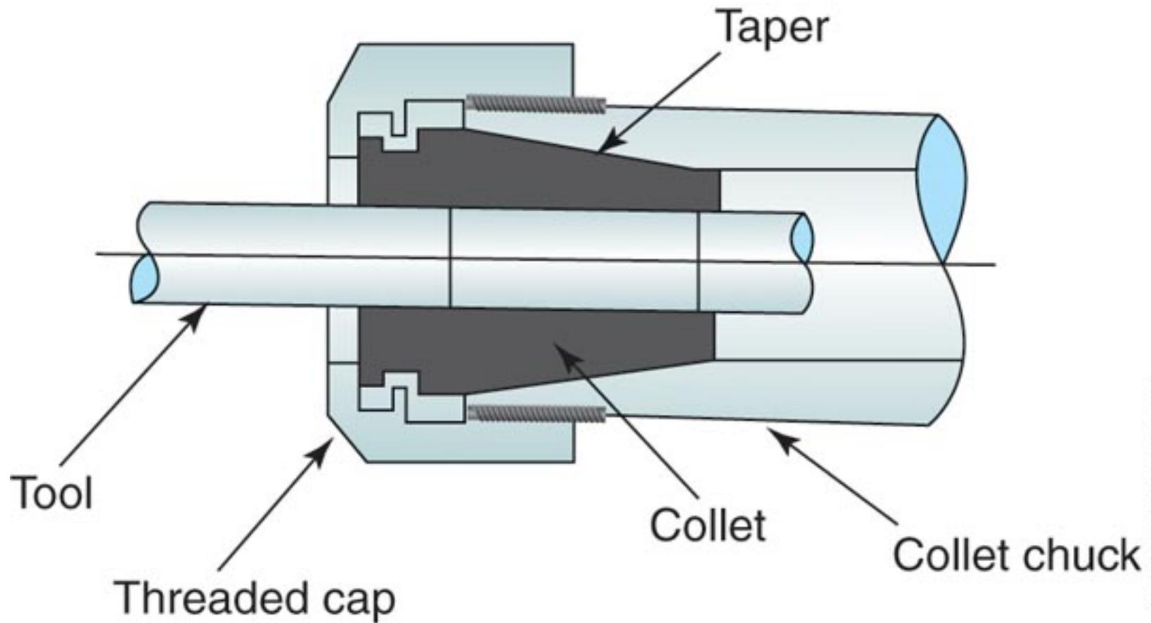
A collet chuck grips a tool shank by tightening the threaded cap.
