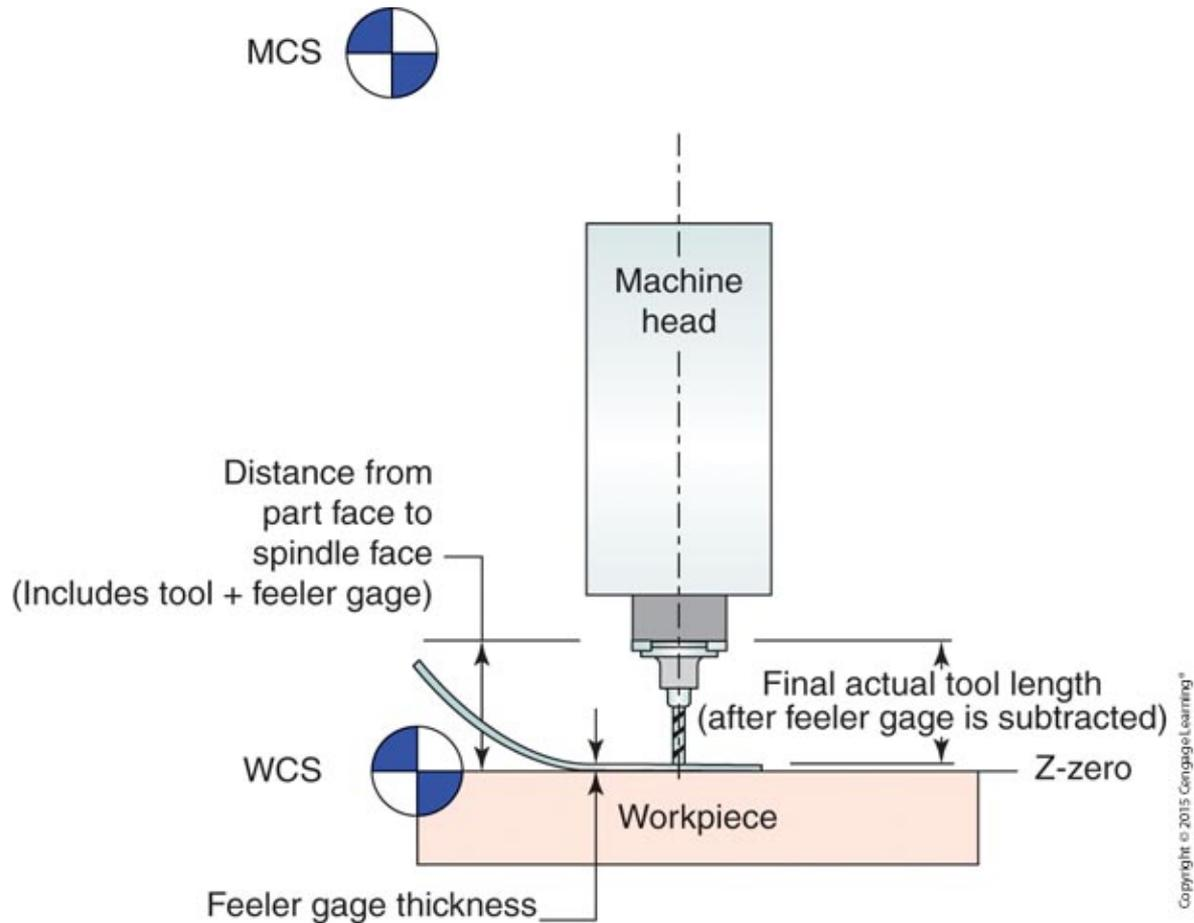
A VMC Z-axis can be used to measure tool length. The length offset is found by touching the tool tip off of the work Z-zero surface with a feeler gage and then subtracting the feeler gage thickness. The objective is to determine the dimension labeled “Final actual tool length.”
