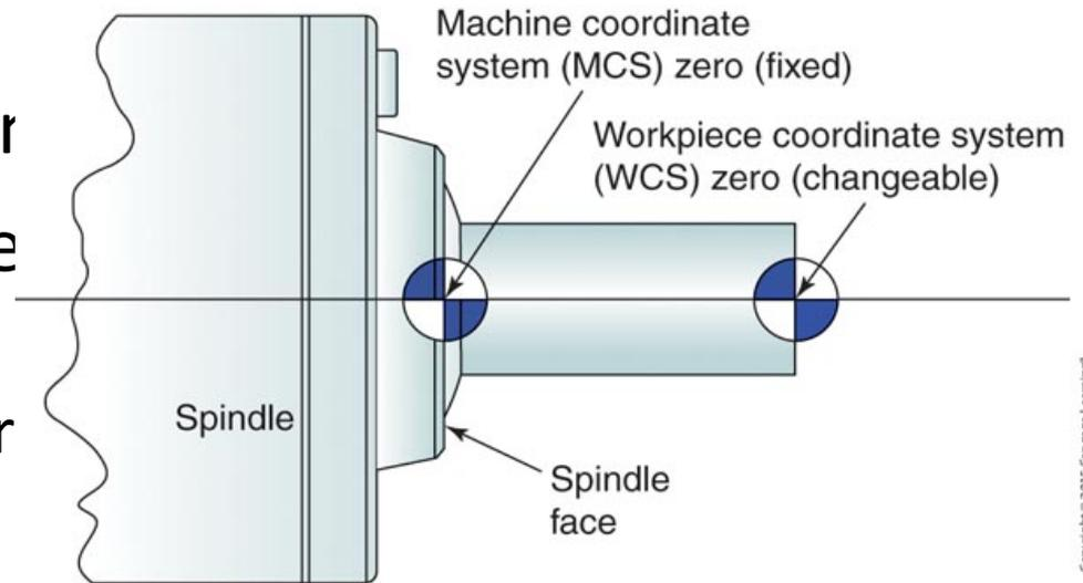
The relationship of the machine coordinate system (MCS) to the established work coordinate system (WCS).
