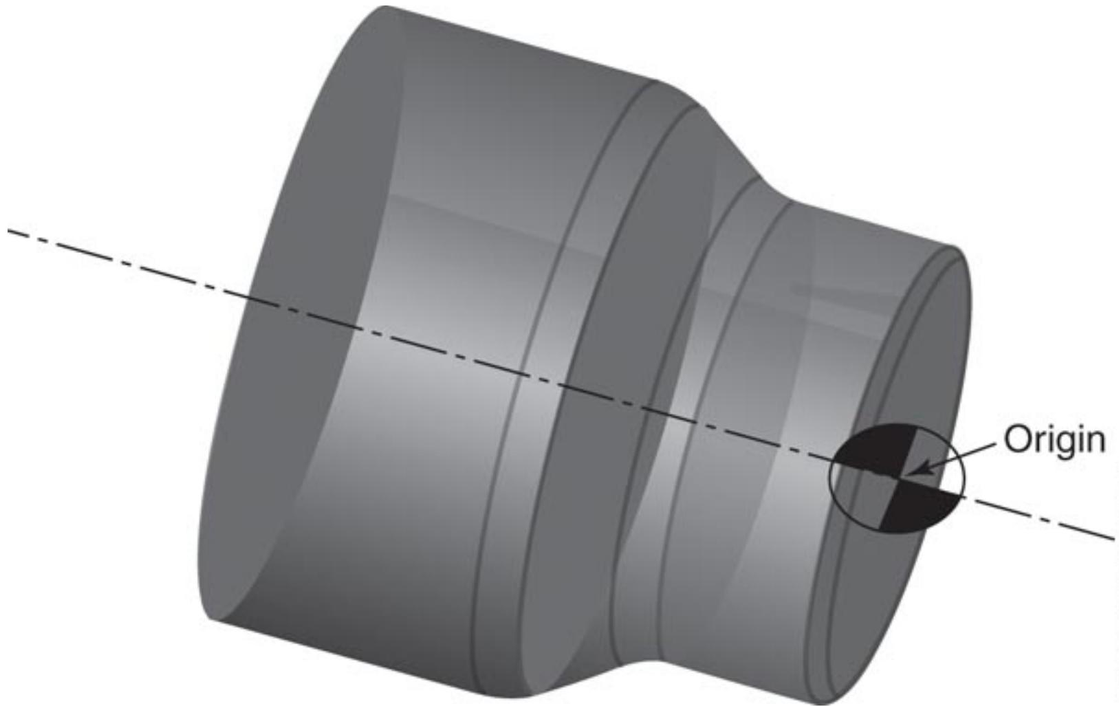
The origin for turning is usually located on the workpiece face on the part center line.
