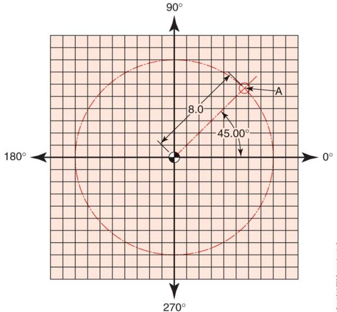
An example of how each position in an eight-hole workpiece can be identified using polar coordinates. The positions for each location are programmed as: (A) X7.0 Y0; (B) X7.0 Y45.0; (C) X7.0 Y 90.0; (D) X7.0 Y135.0; (E) X7.0 Y180.0; (F) X7.0 Y225.0; (G) X7.0 Y270.0; (H) X7.0 Y315.0
