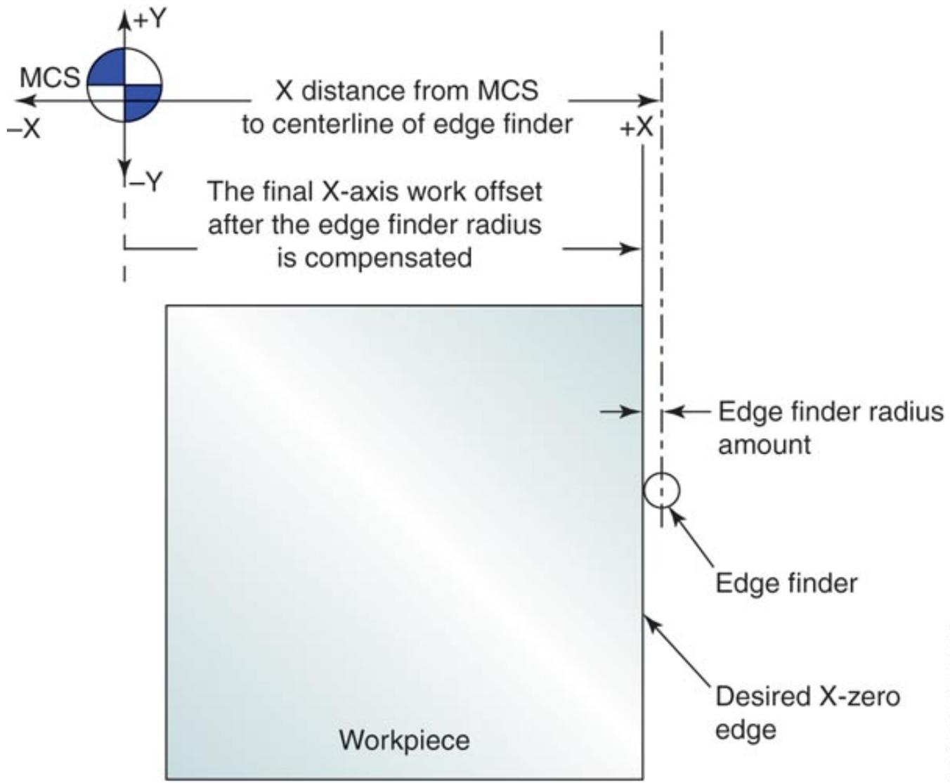
Right-edge workpiece X-zero work offset
