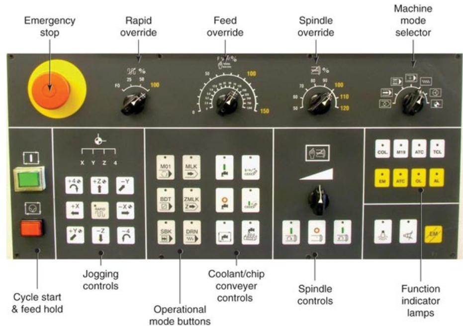
The parts of a machining center control panel.
