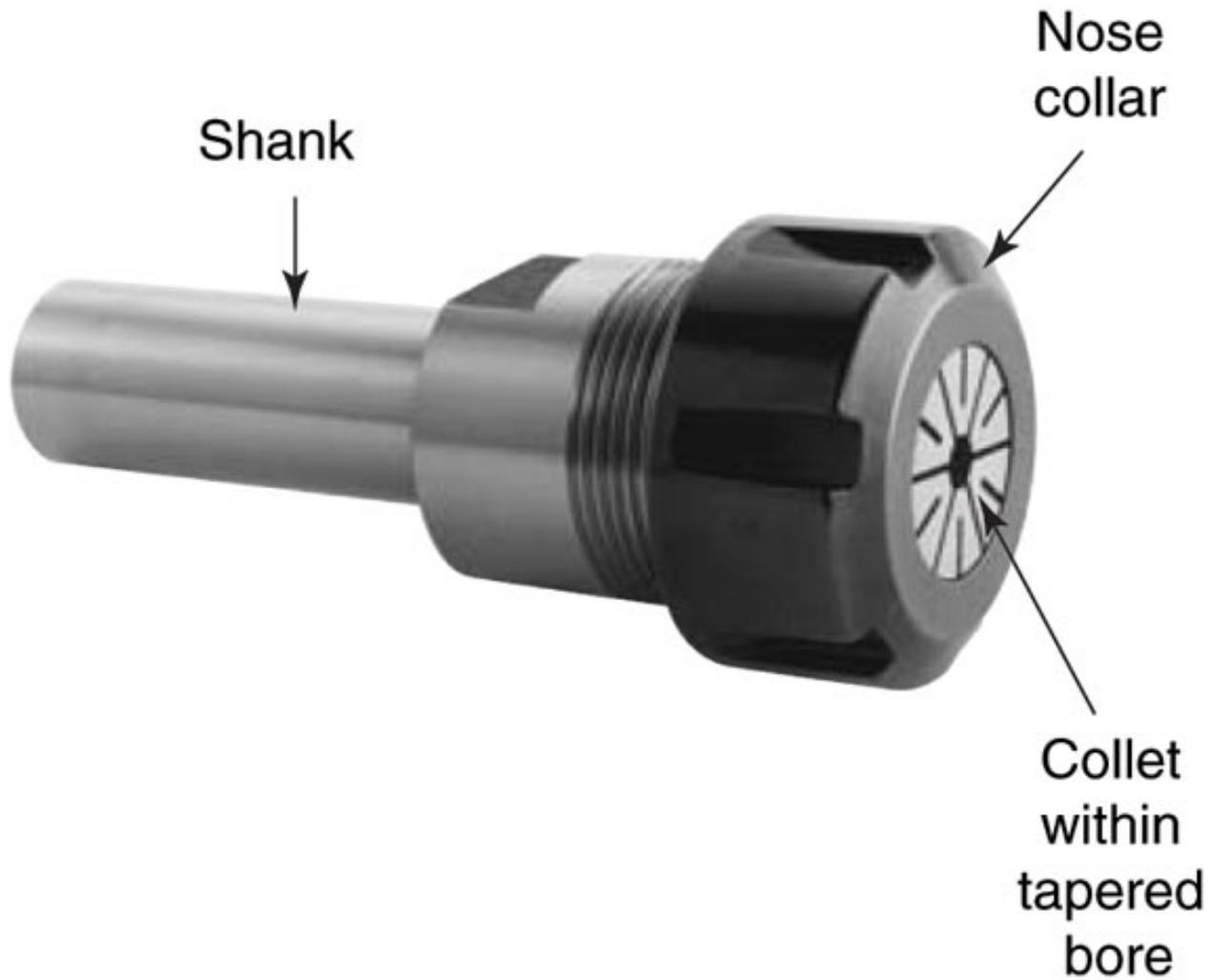
A CNC collet chuck for holding holemaking tools.
