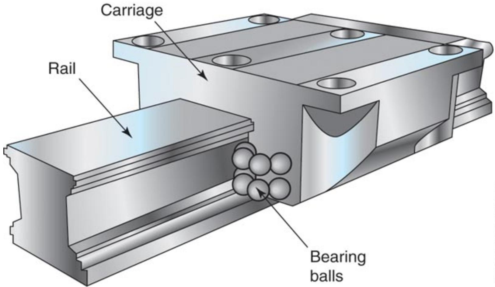
A linear guide assembly and its parts.
