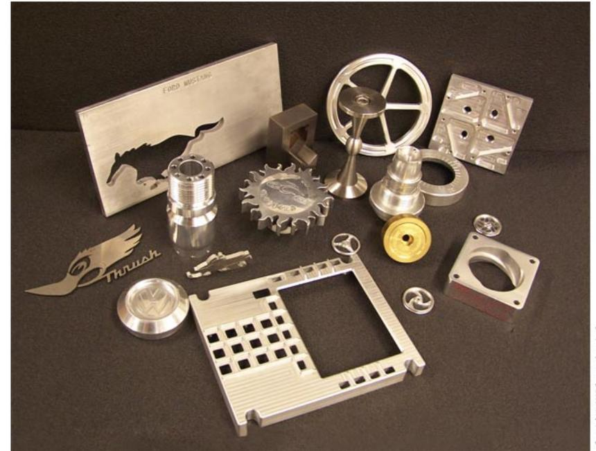
Examples of some workpieces produced by CNC machines.
