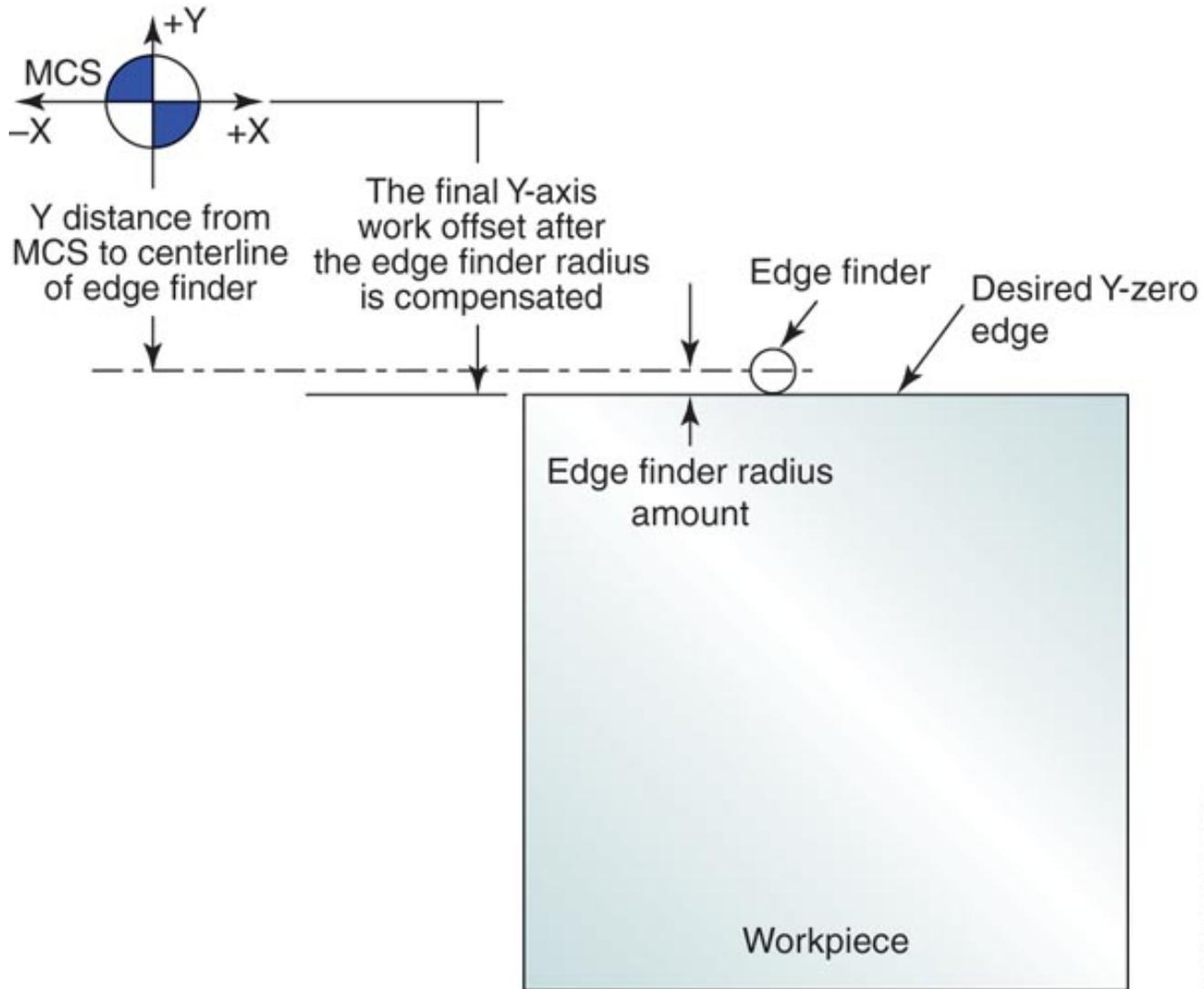
Rear-edge workpiece Y-zero work offset
