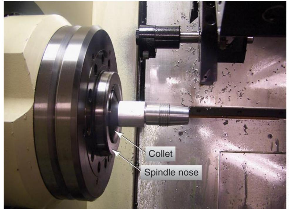
A CNC turning center using a collet for workholding.
