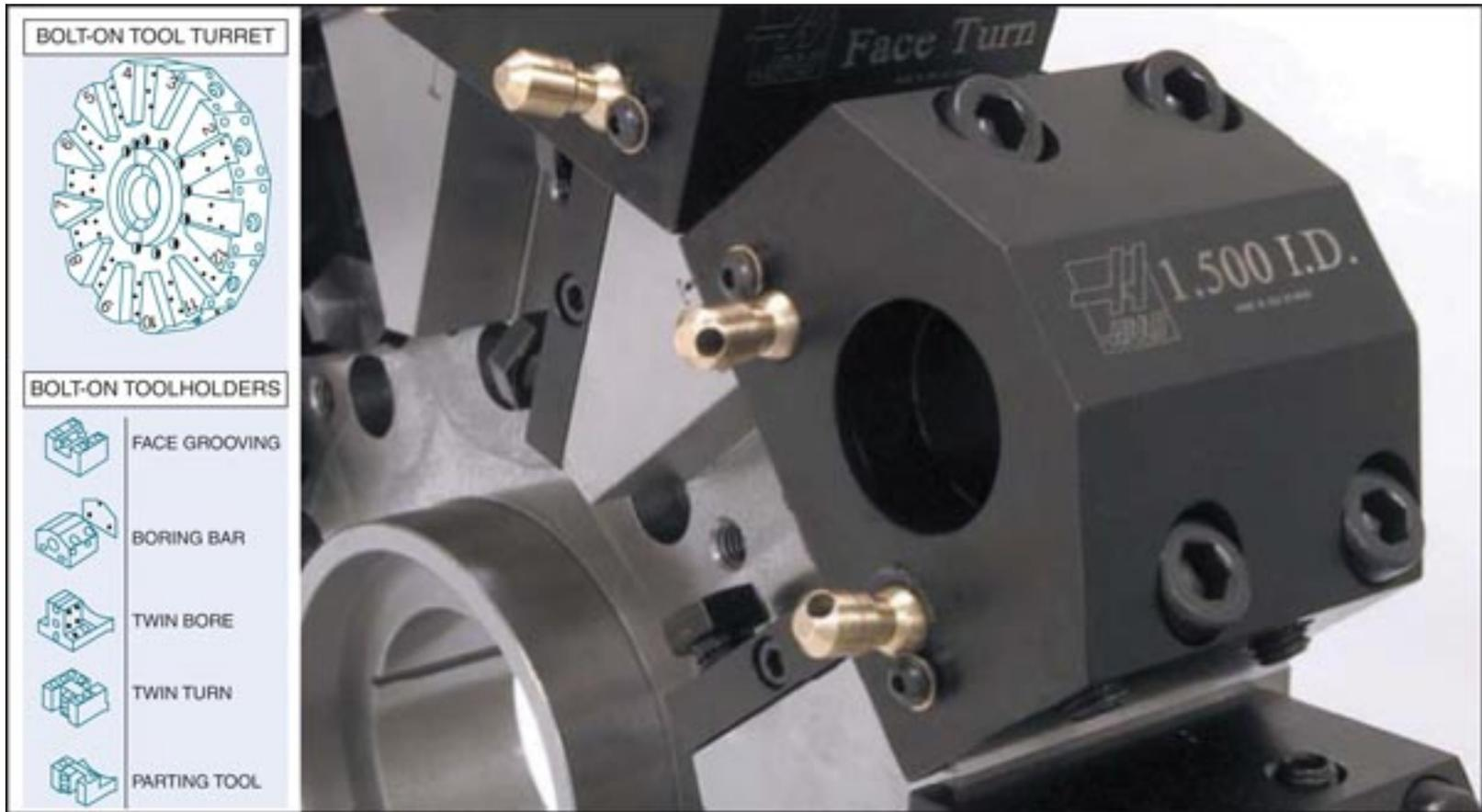
This type of toolholding adapter bolts directly to the turret with cap screws..
