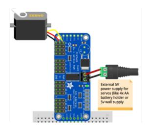
Servo orange wire to breakout PWM on channel 0 Servo red wire to breakout V+ on channel 0 Servo brown wire to breakout Gnd on channel 0 Check your servo data sheet to verify how to connect it!
