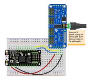
Board 3V to driver VCC Board GND to driver GND Board SCL to driver SCL Board SDA to driver SDA
