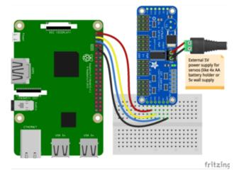
Pi 3V3 to driver VCC Pi GND to driver GND Pi SCL to driver SCL Pi SDA to driver SDA
