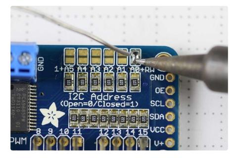
Board 0: Address = 0x40 Offset = binary 00000 (no jumpers required) Board 1: Address = 0x41 Offset = binary 00001 (bridge A0 as in the photo above)
