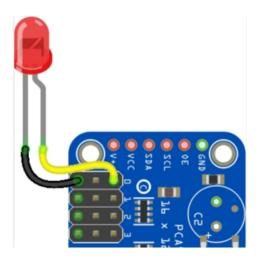
LED cathode / shorter leg to PCA9685 channel GND / ground. LED anode / longer leg to PCA9685 channel PWM.
