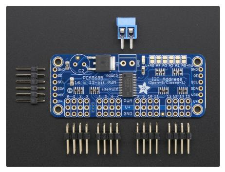
There are two sets of control input pins on either side. **Both sides of the pins are identical!** Use whichever side you like, you can also easily chain by connecting up two side-by-side
