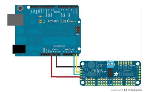
The VCC pin is just power for the chip itself. If you want to connect servos or LEDs that use the V+ pins, you MUST connect the V+ pin as well. The V+ pin can be as high as 6V even if VCC is 3.3V (the chip is 5V safe). We suggest connecting power through the blue terminal block since it is polarity protected.
