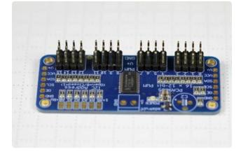
Install the Servo Headers Install 4 3x4 pin male headers into the marked positions along the edge of the board.
